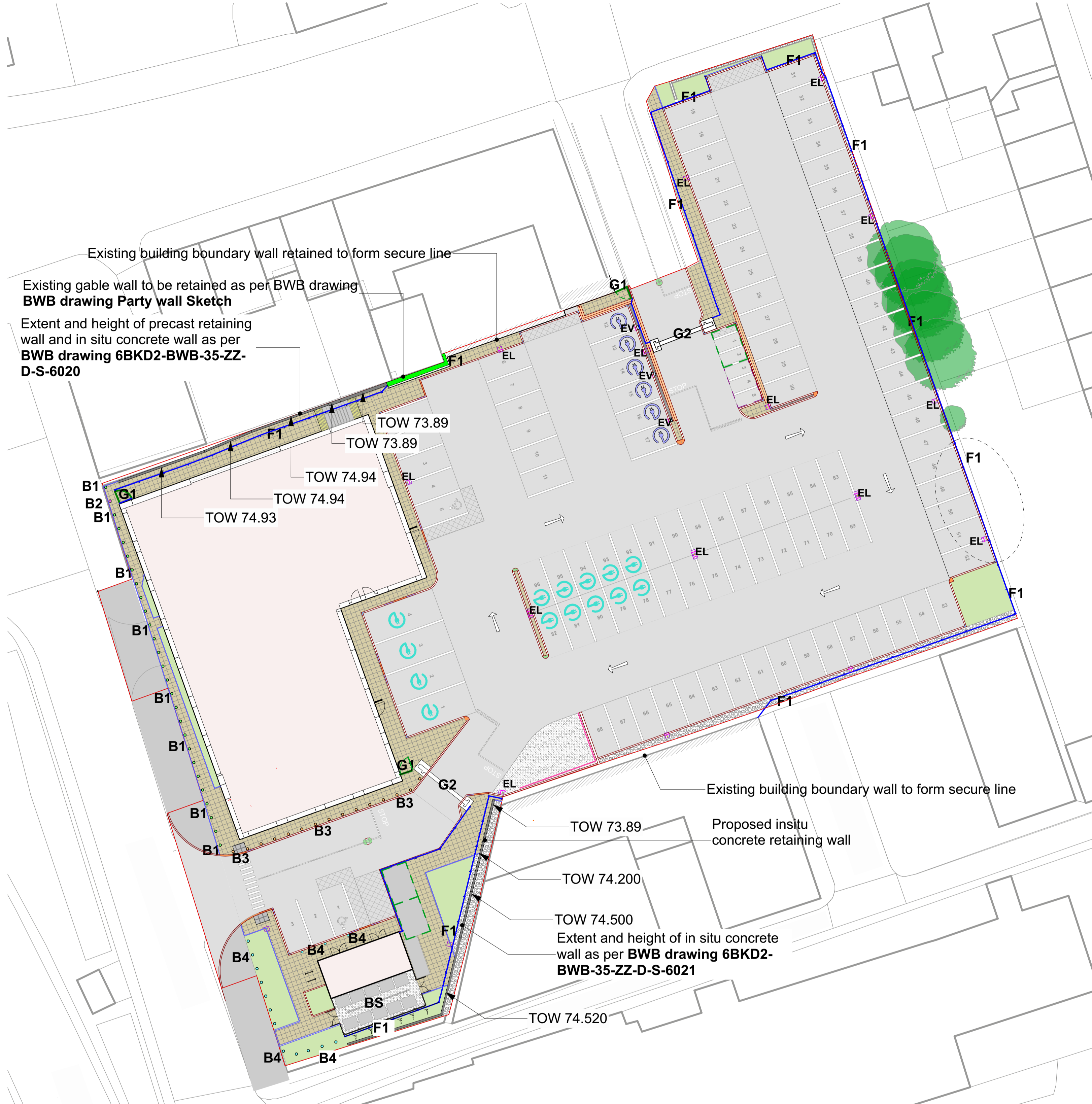
G1- 1.2m wide single leaf Pedestrian Gates UHS Extreme Mesh SR3 Height Overall to line through with fence to maintain perimeter security - over panel may be required
