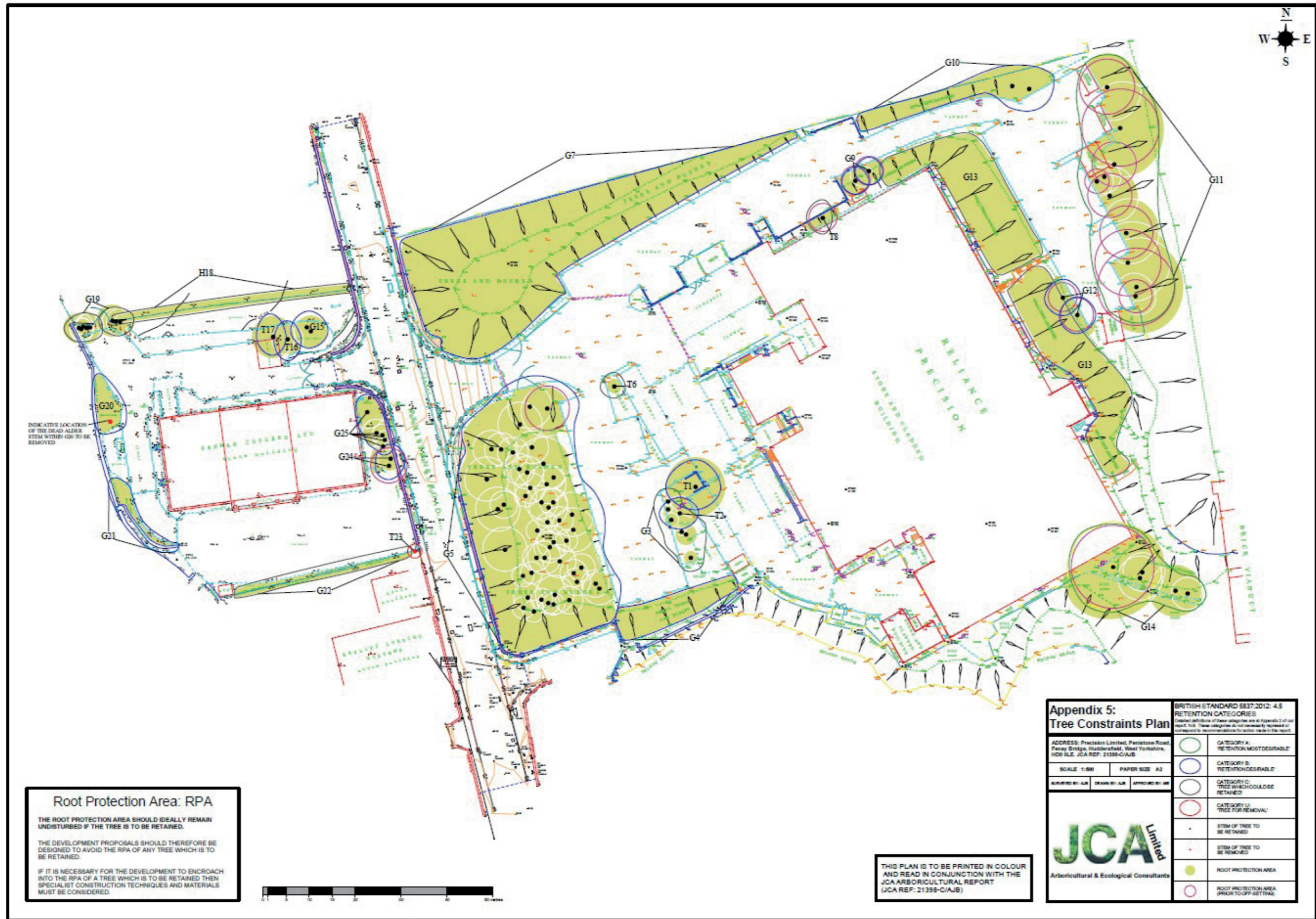
APPENDIX 3: Tree Constraints Plan from 'Arboricultural Impact Assessment' by JCA Ltd Arboricultural & Ecological Consultants (2025)
