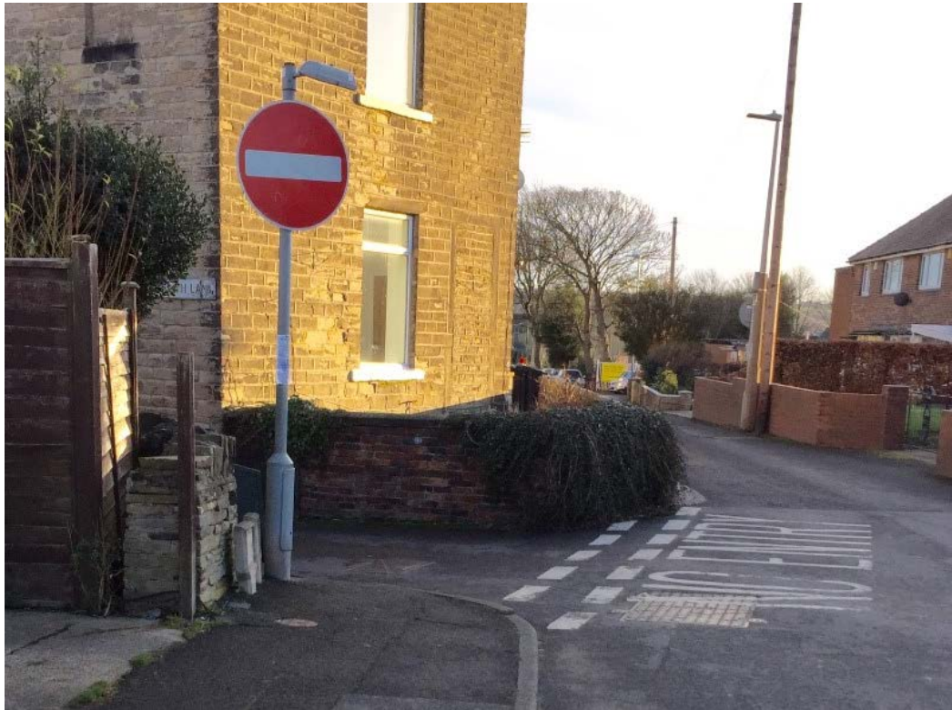
Photo 3. Hepworth Lane Junction With Wellhouse Lane – Visibility to the Left Almost Zero
