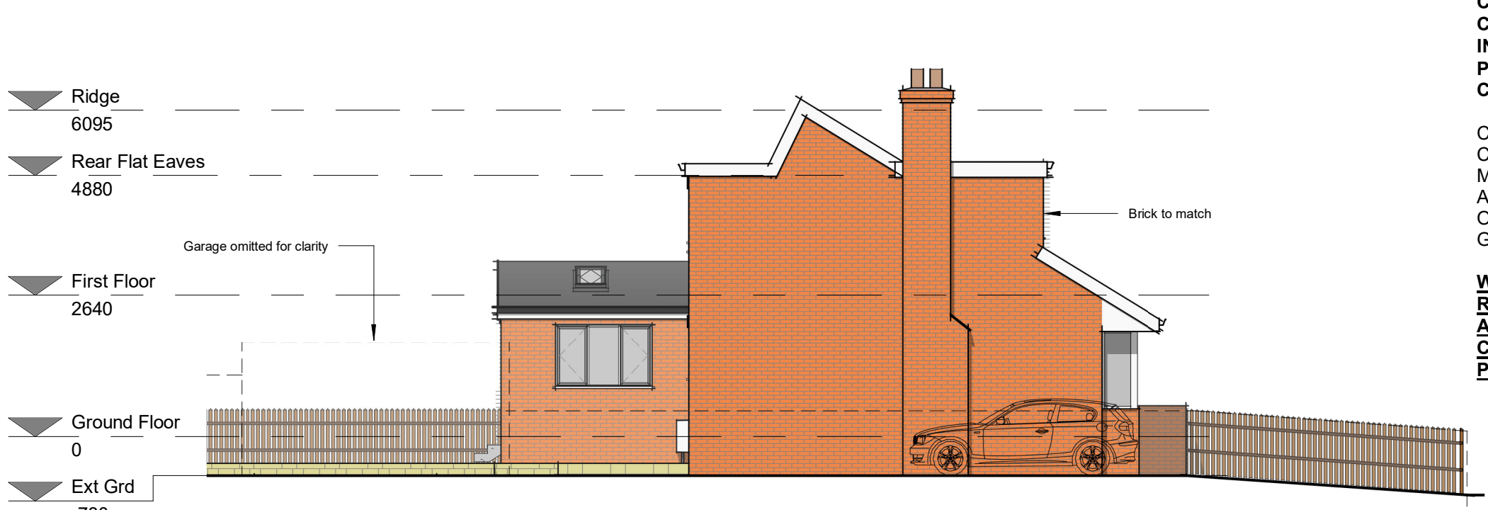
Side Elevation (South Facing) 1 : 100
