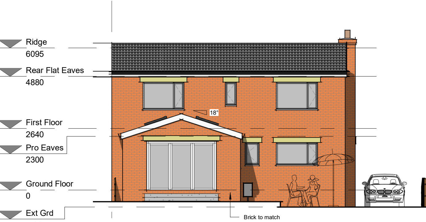
Rear Elevation (West Facing) 1 : 100
