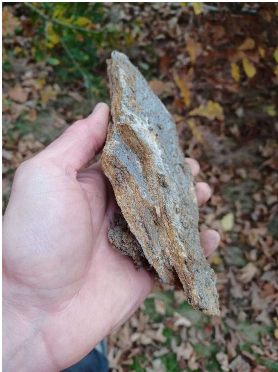
Photograph 5: Texture of the sandstone recovered from a depth of 0.50 m below ground level in TP106
