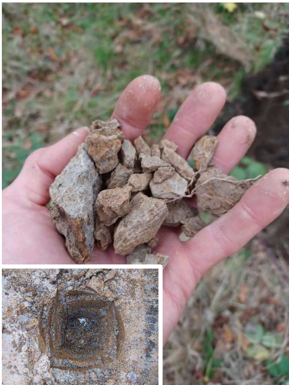
Photograph 6: Texture of the siltstone (and inferior sandstone) recovered from a depth of 1.00 m below ground level in TP101
