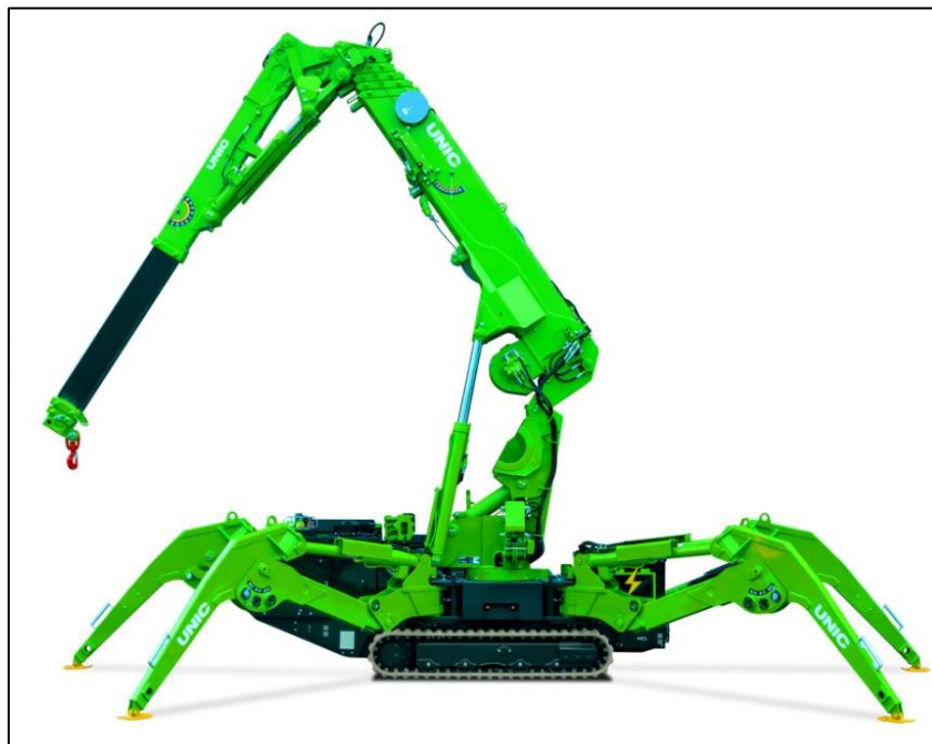
Figure 15: Typical spider crane
