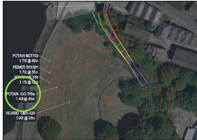
Figure 7 – Tower crane location and lifting radius
