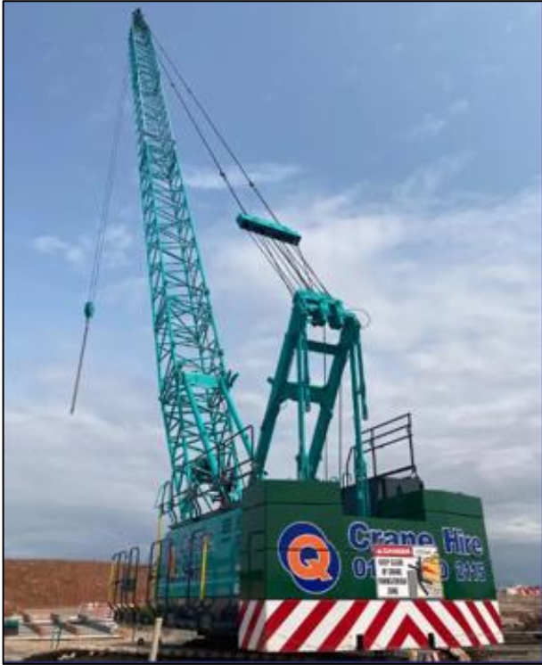
Figure 8 – Typical 90T crawler crane
