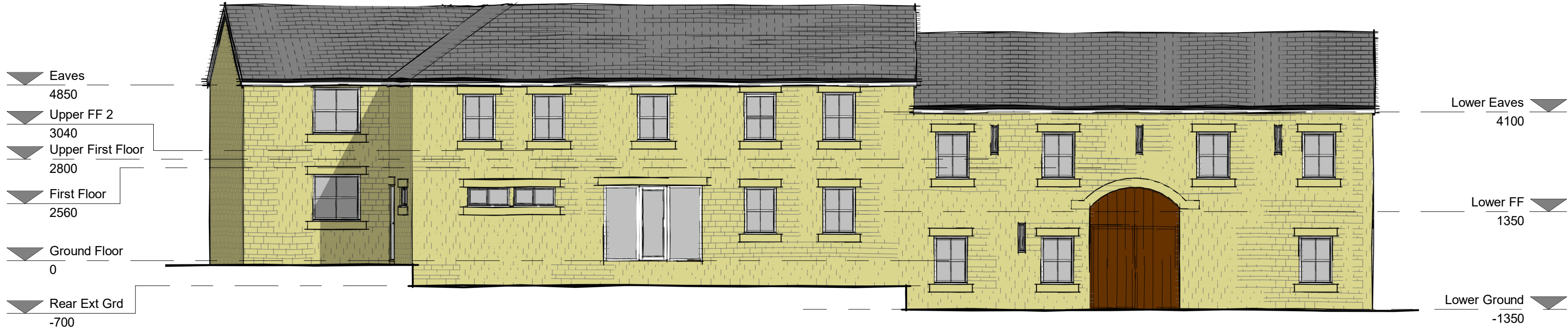
Rear Elevation (SE Facing) 1 : 100
