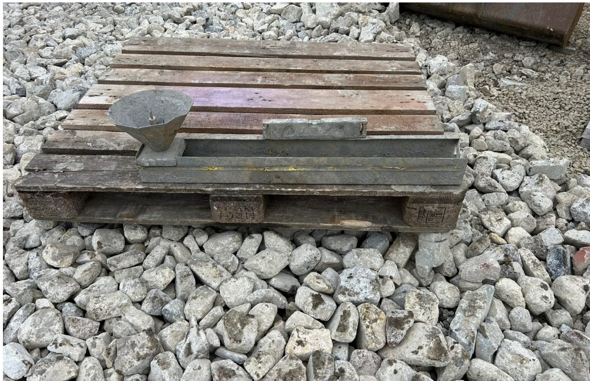
Photograph 6 – Photograph of grout flow testing equipment.
