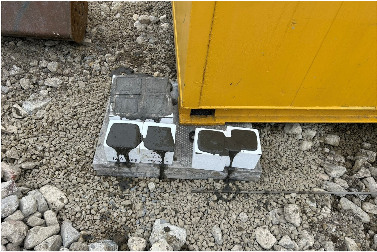
Photograph 5 – Photograph of grout cubes gathered during the works
