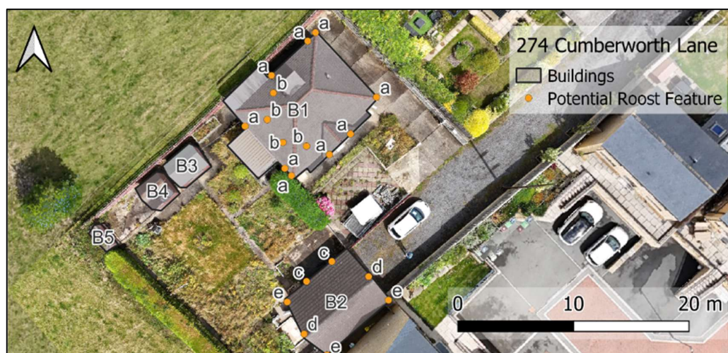
Figure A5.1. Potential bat roost features identified during the inspection
