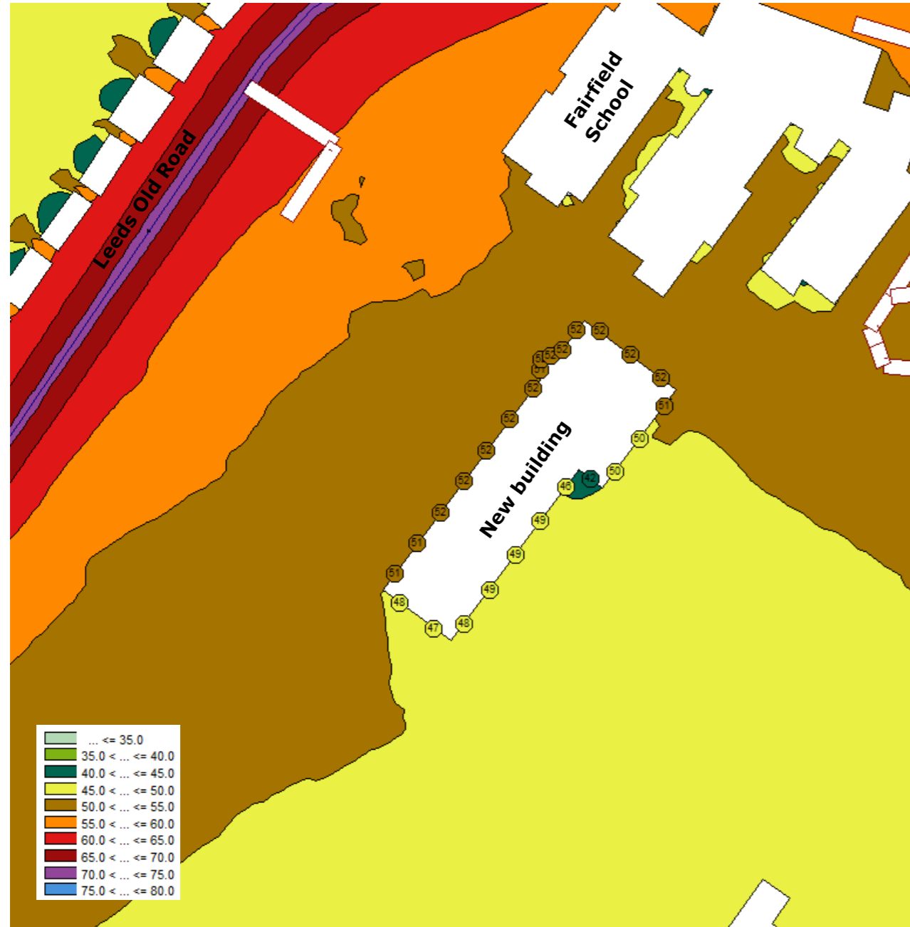
Figure 2 – Noise map based on levels from Ramboll noise survey, LAeq, 30min at 1.5m height.
