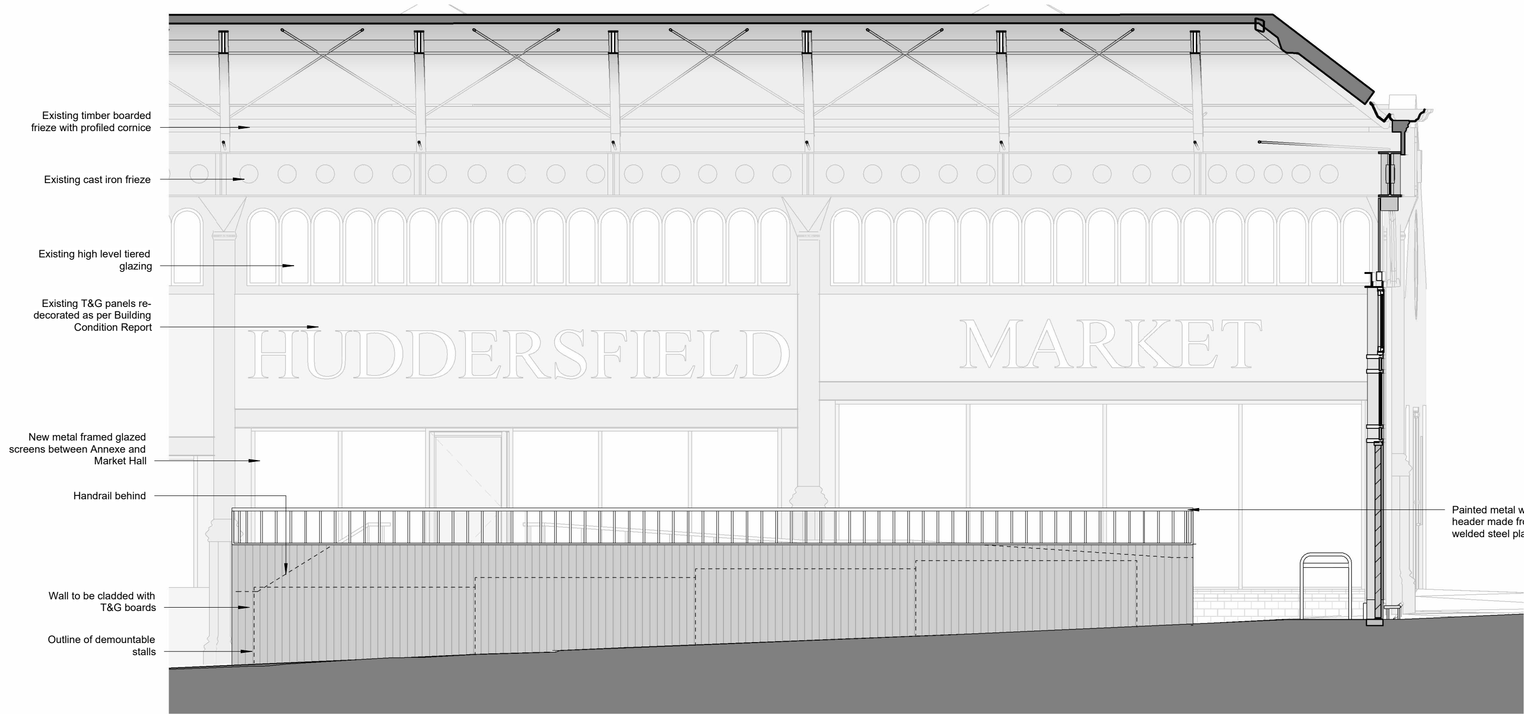
2 Warm Box Commercial Kitchen and Bar - Elevation 1 : 50
