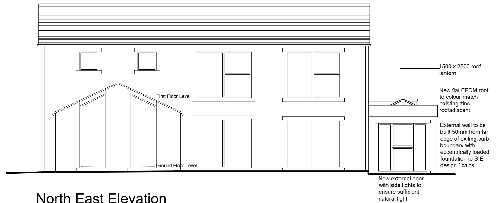
North East Elevation (rear)
