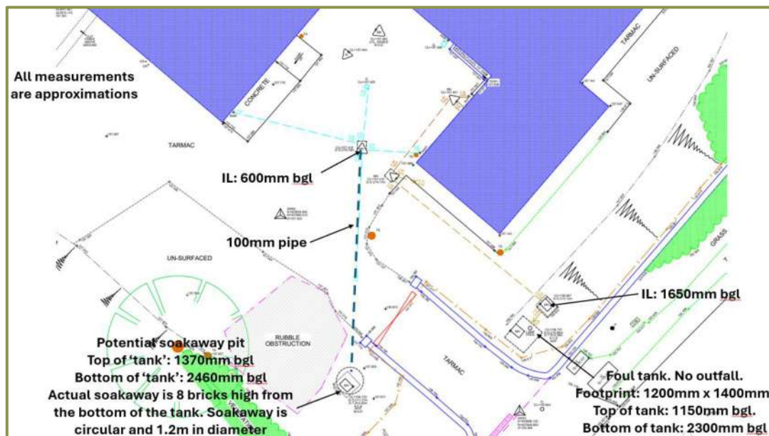
Figure 4.2: CCTV Survey Findings
