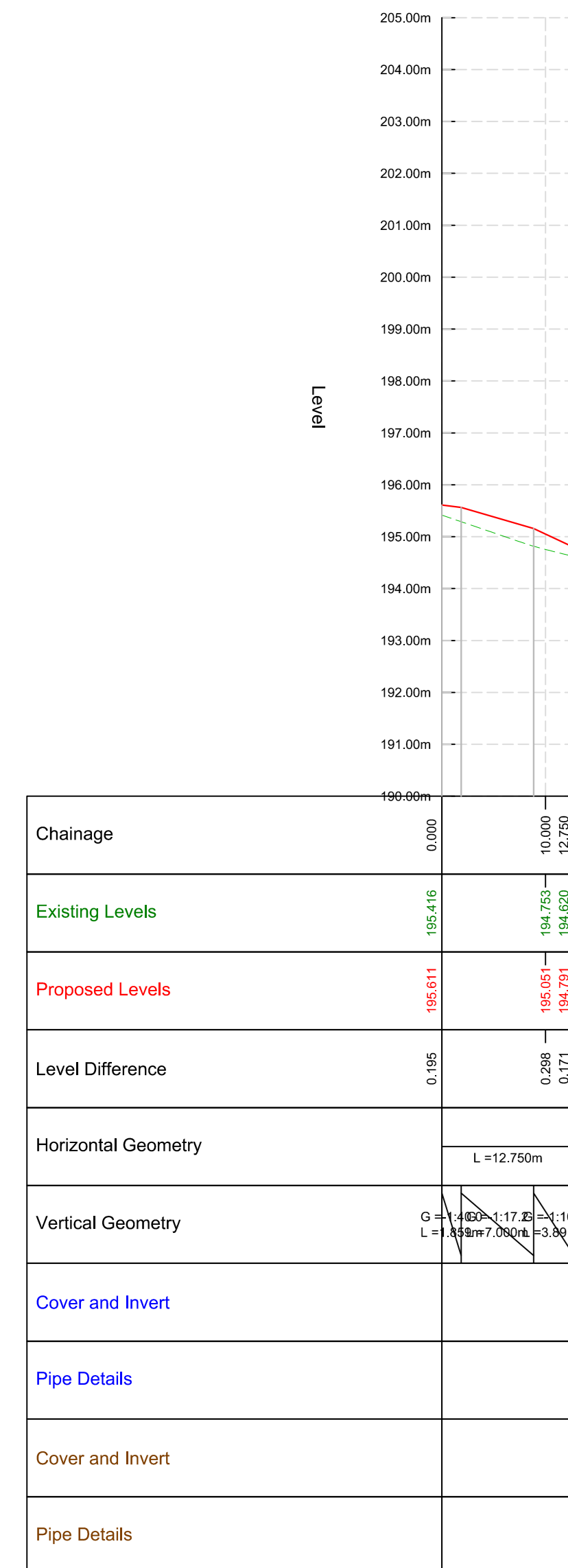
ROAD 04 - LONGSECTION Scale: H 1:500,V 1:100. Datum: 190.000
