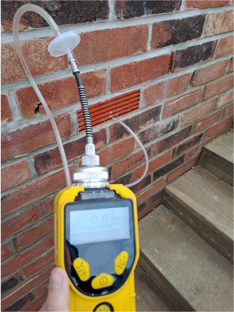
Photo 6 : PID in operation. 05/03/2025
