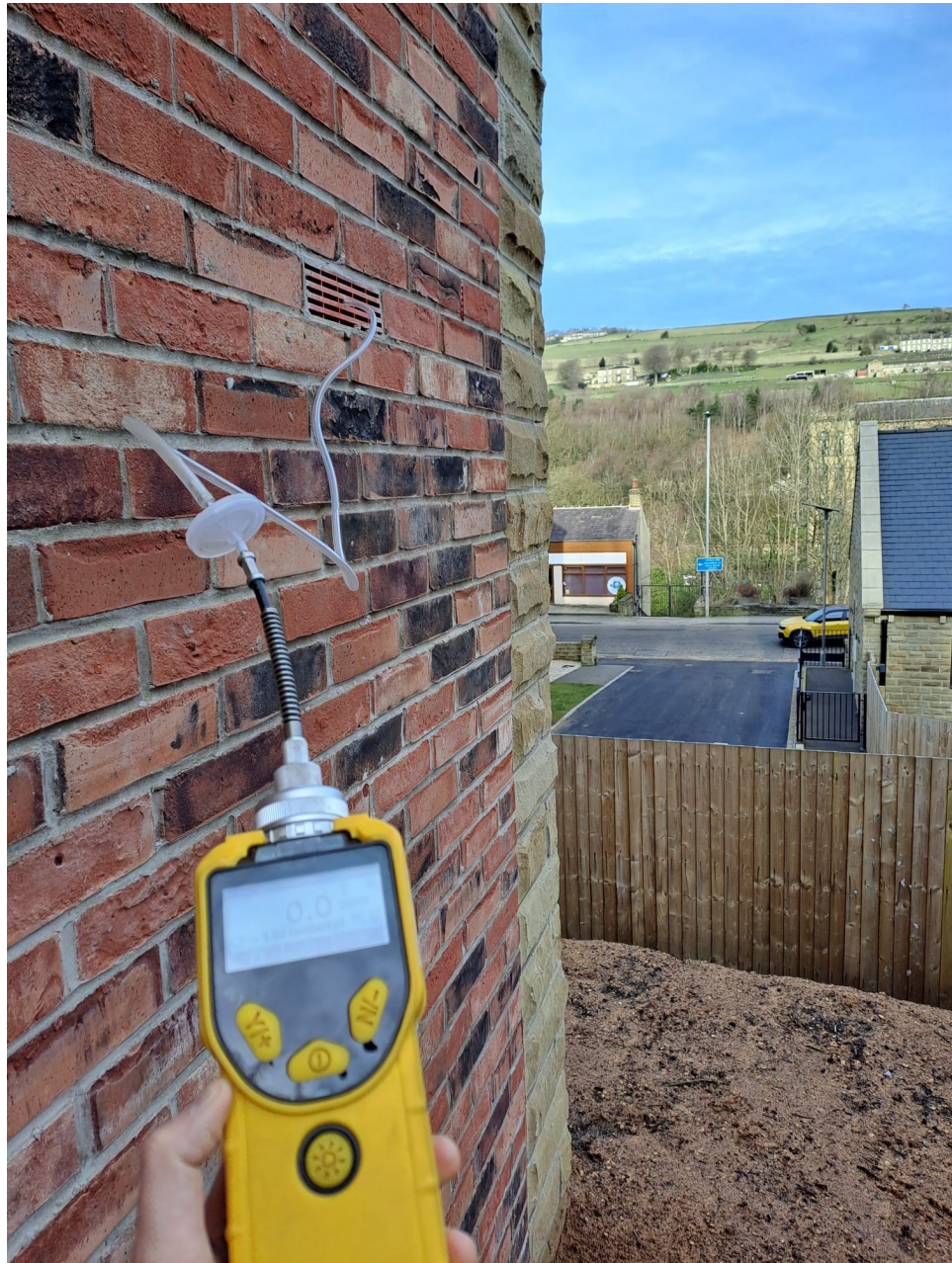
Photo 7 : PID in operation. 05/03/2025
