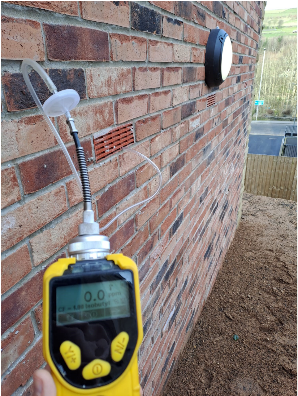
Photo 5 : PID in operation. 05/03/2025
