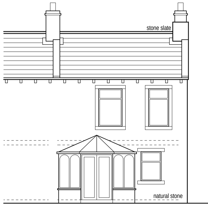
Existing rear/north west facing elevation (1:100)
