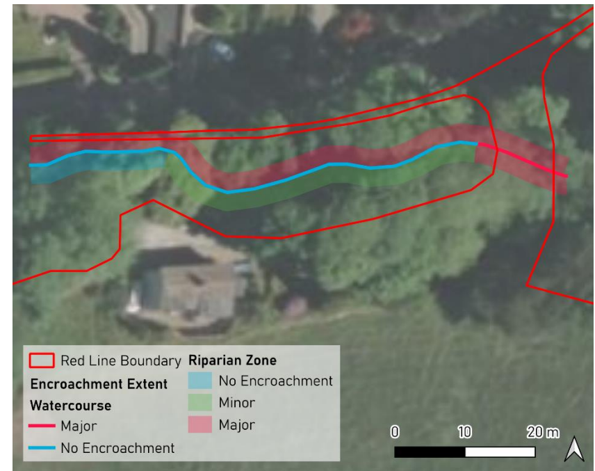
Figure 10 Encroachment assessment of Ludhill Dike.
