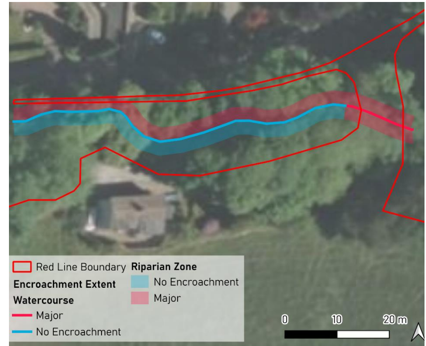
Figure 11 Post-development encroachment assessment of Ludhill Dike.
