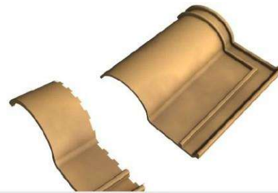
Tiles cutting for top flashing
