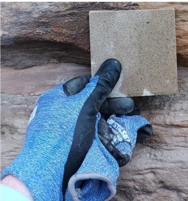
Insert 1 Sample of Crosland Hill sandstone held against historic stonework of Huddersfield Viaduct (MVL3/92) (left), with masonry of Wood Lane Overbridge (MDL1/23) (right).
