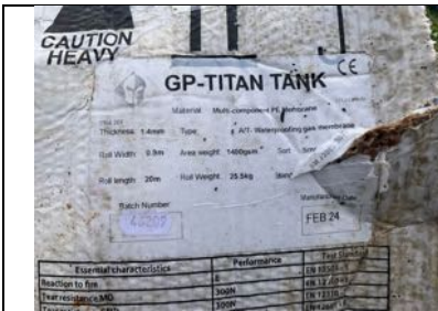
Evidence of the Juta TitanTank membrane used on this project.
