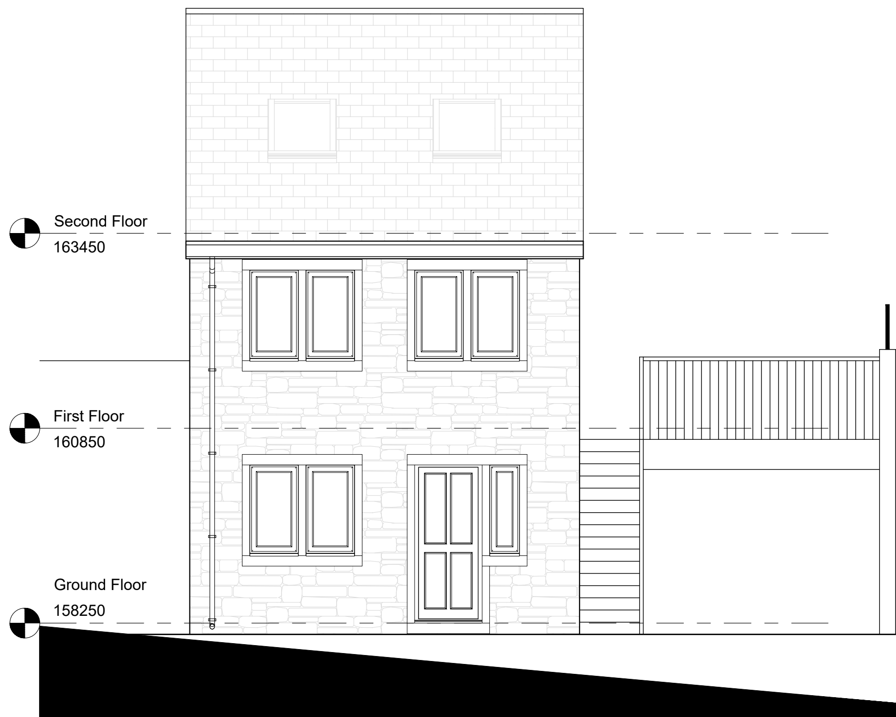
1 PROPOSED SOUTH-WEST ELEVATION SCALE 1:50
