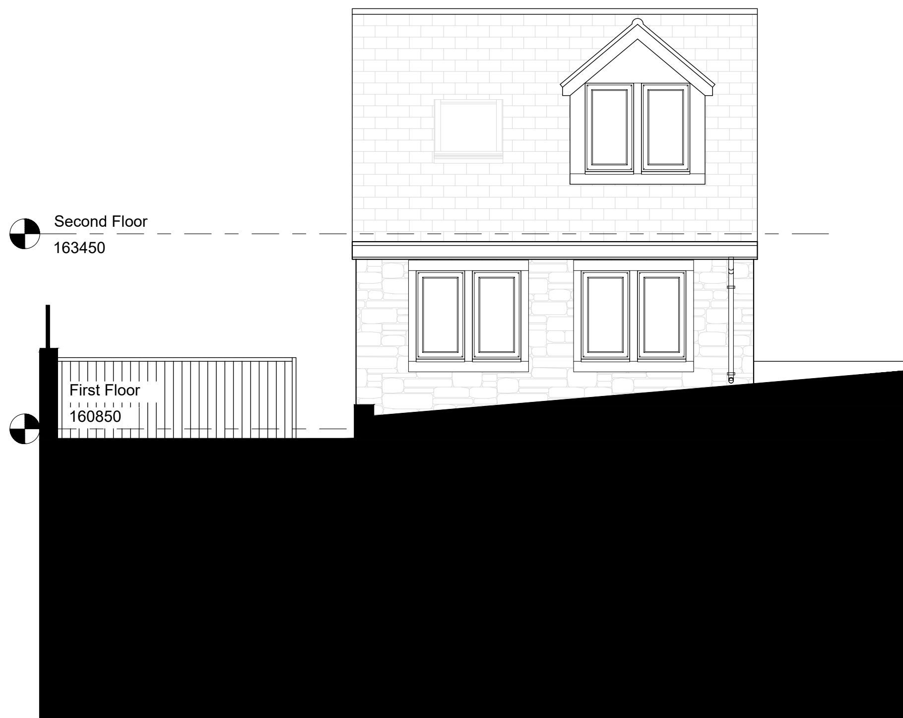
3 PROPOSED NORTH-EAST ELEVATION SCALE 1:50
