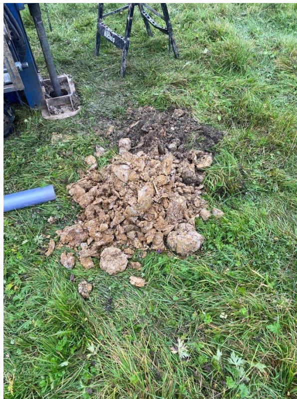
Photograph 4: Arisings from the hand pit of BH005R(S) to 1.20 m begl.
