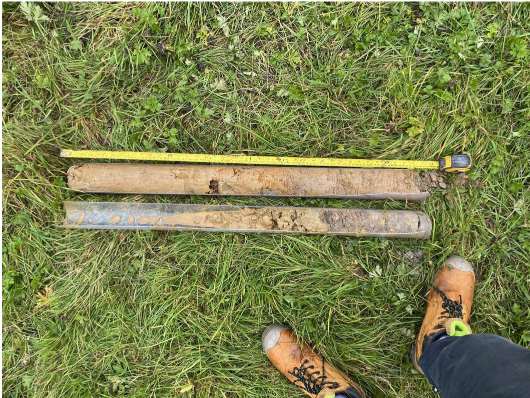
Photograph 5: Arisings from BH005R(S) between 1.00 – 2.50 m begl.
