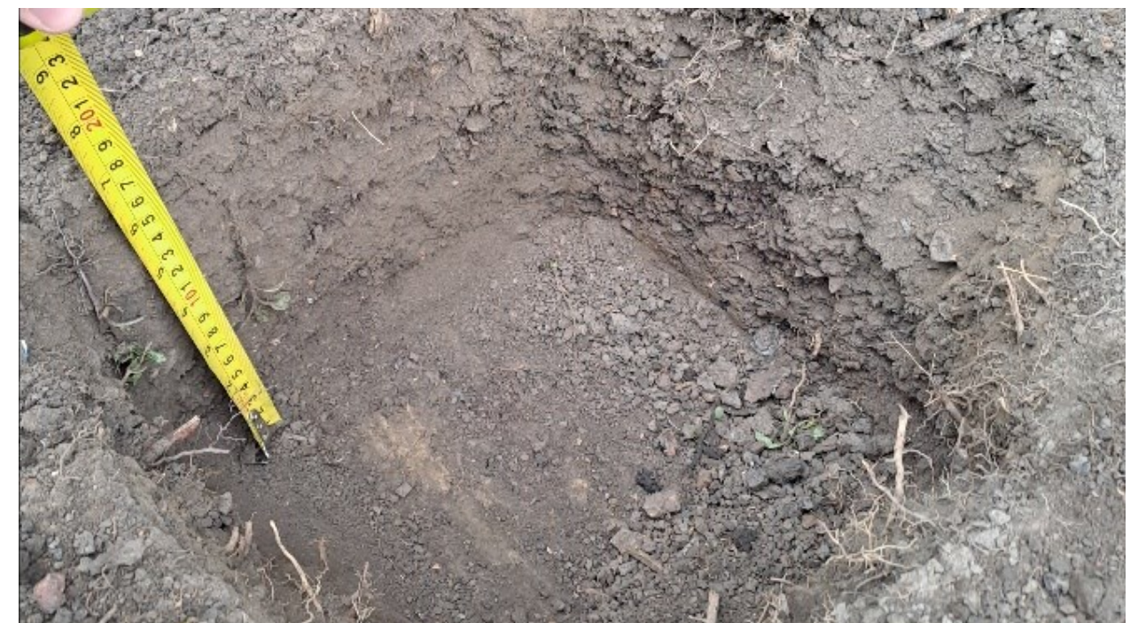
Photo 2: Cross section near building which shows nominal thickness of topsoil above natural soil.
