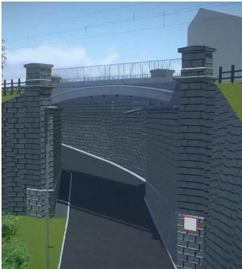
Insert 3-6 Visualisation of the proposed western elevation of Jack Lane Underbridge (MDL1/24), from the south-west. Note, as above, the fascia arch beam will be painted green and white (see accompanying Materials Schedule and LBC drawings).
