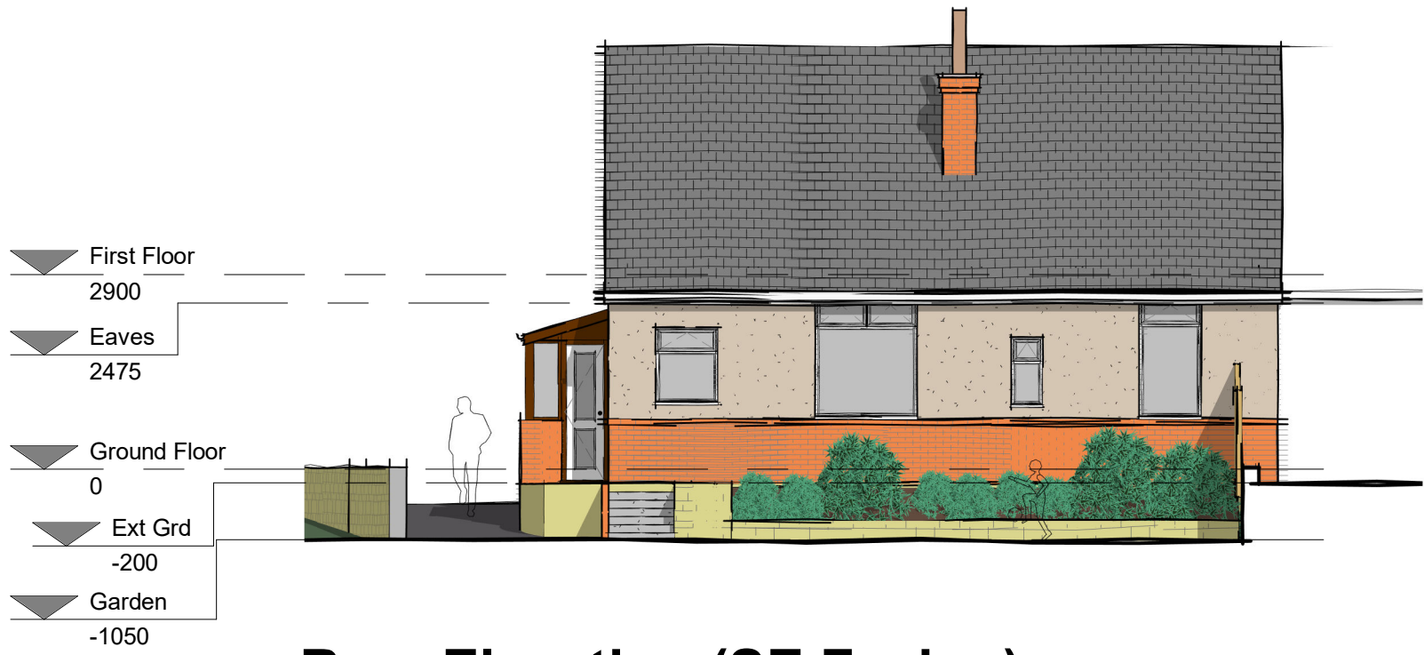
Rear Elevation (SE Facing) 1 : 100
