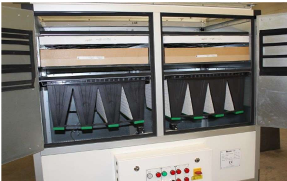
Fig No. 63. The picture below shows a separate recirculation unit. In this case the model shown is manufactured by Reco-Air. ( www.reco-air.com )
