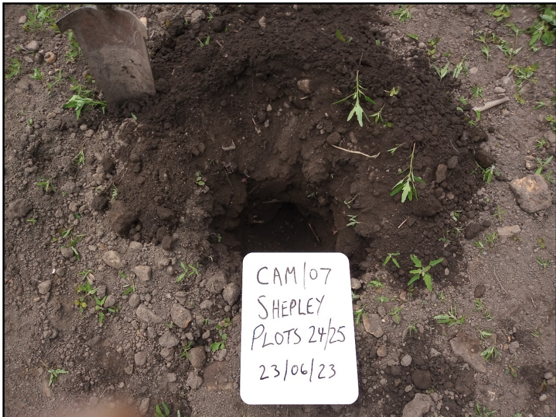
Plots 24/25: Hard break of crushed brick and stone at base of cover.
