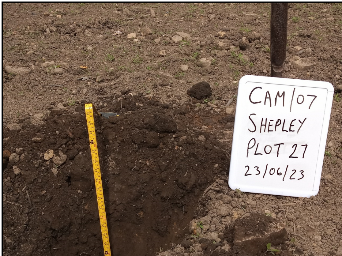
Plot 27: Clean cover validation pit, tube removed, 0.6m depth achieved.
