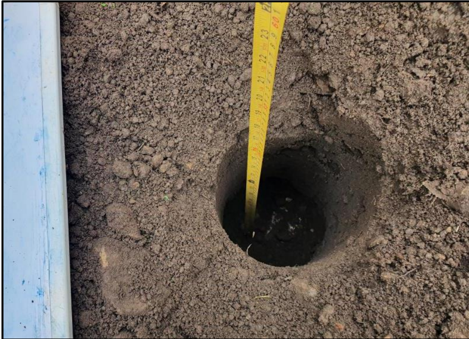
Plot 12: Tube pulled out and clean cover inspected. Hardbreak at the base of the cover.
