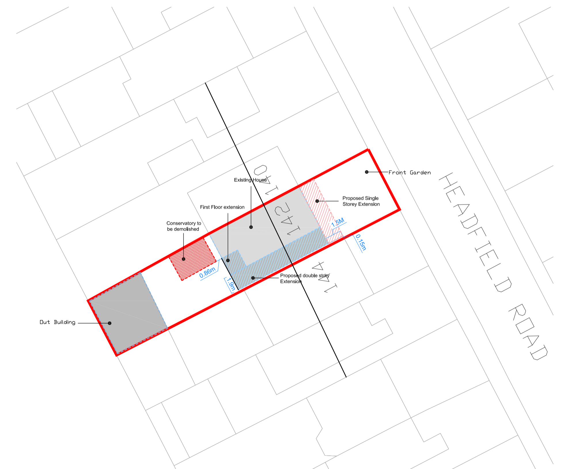
PROPOSED SITE PLAN Scale 1:250@A1
