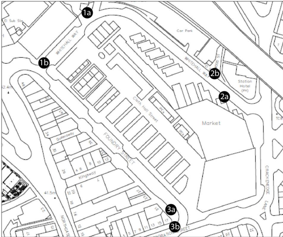
Figure 2: Existing site plan indicating noise monitoring locations
