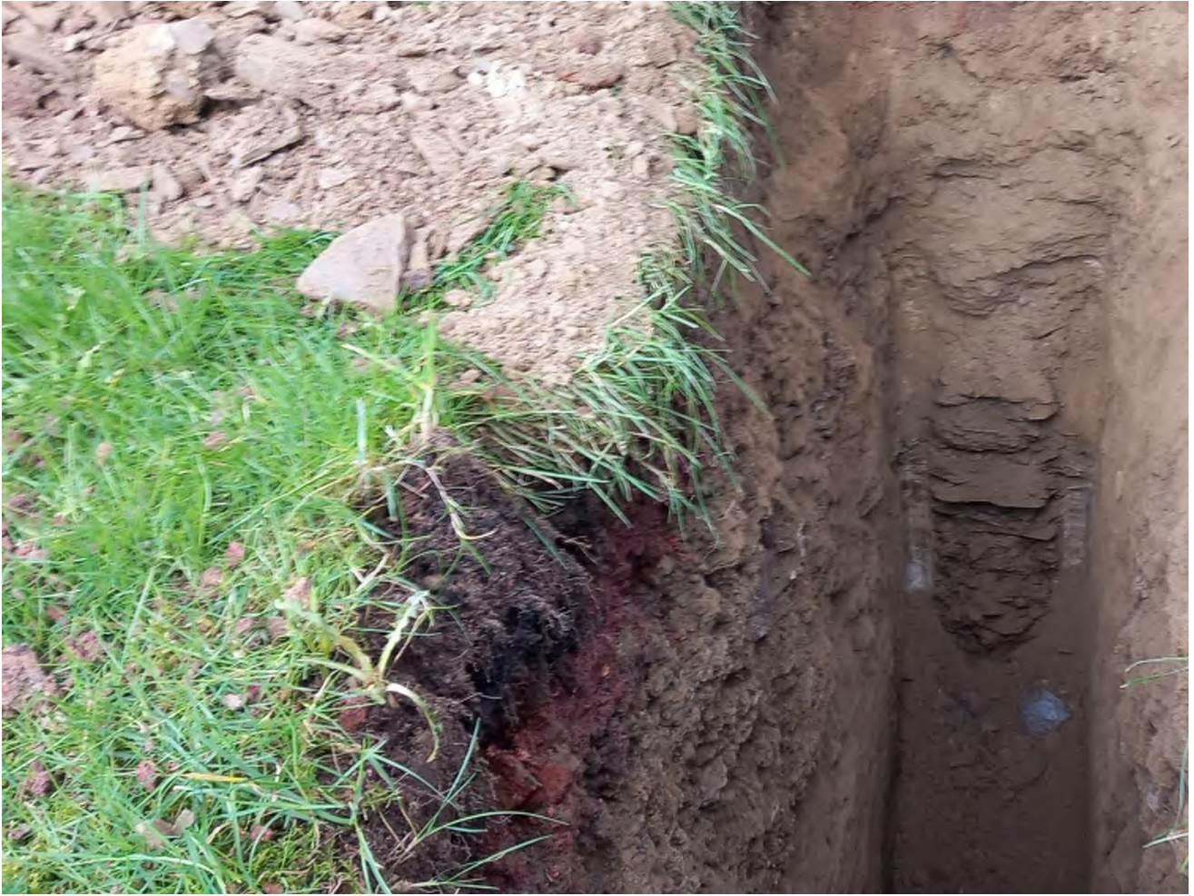
24/02/26 Photo 35 SA201. width 600mm x length 1700mm Topsoil 0.3m over made ground red shale to 0.4m over laminated siltstone bedrock to 1.5m.
