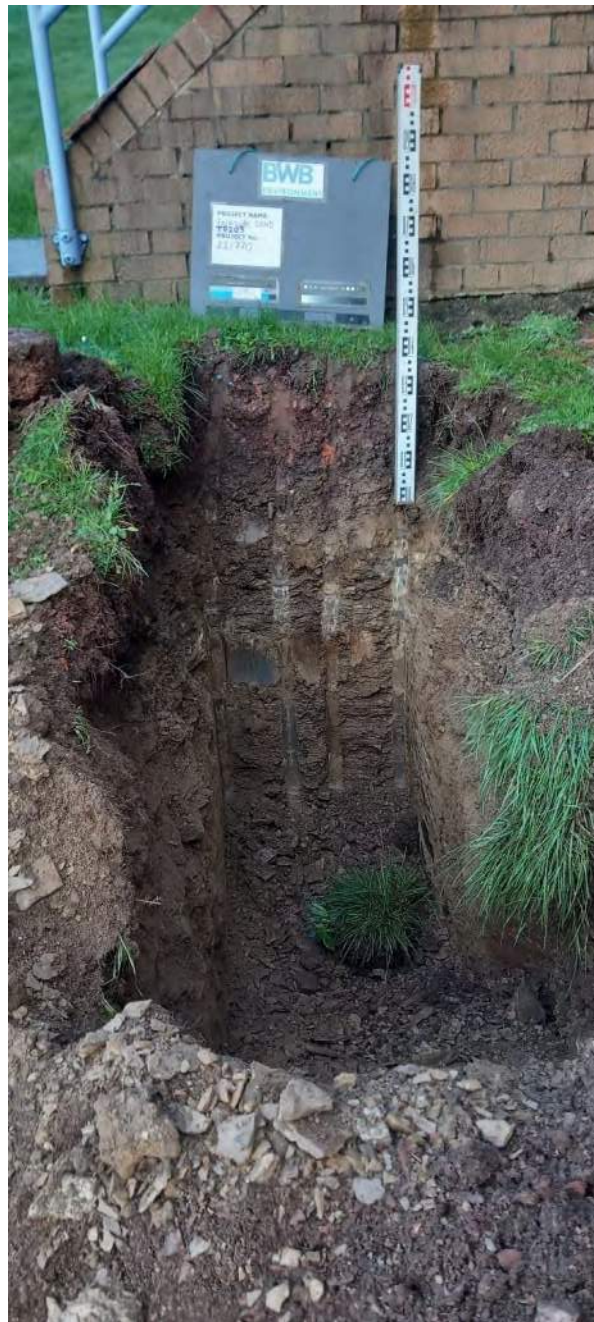
24/02/23 Photo 19 TP203. Topsoil with some bricks over Weathered bedrock
