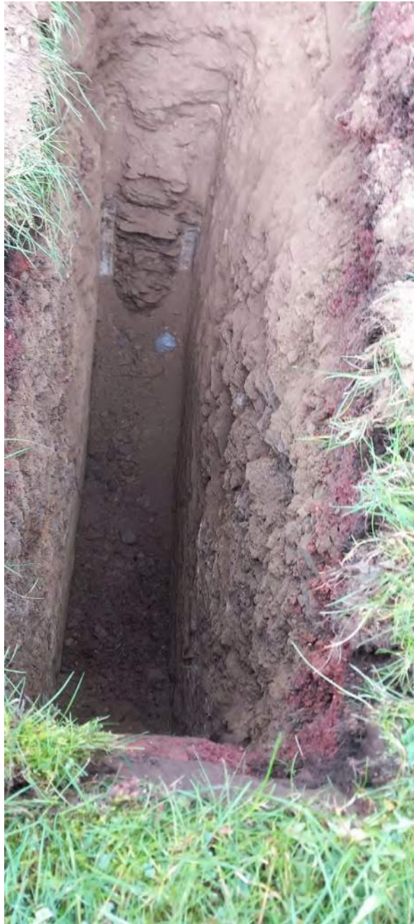
24/02/26 Photo 34 SA201. width 600mm x length 1700mm Topsoil 0.3m over made ground red shale to 0.4m over laminated siltstone bedrock to 1.5m.
