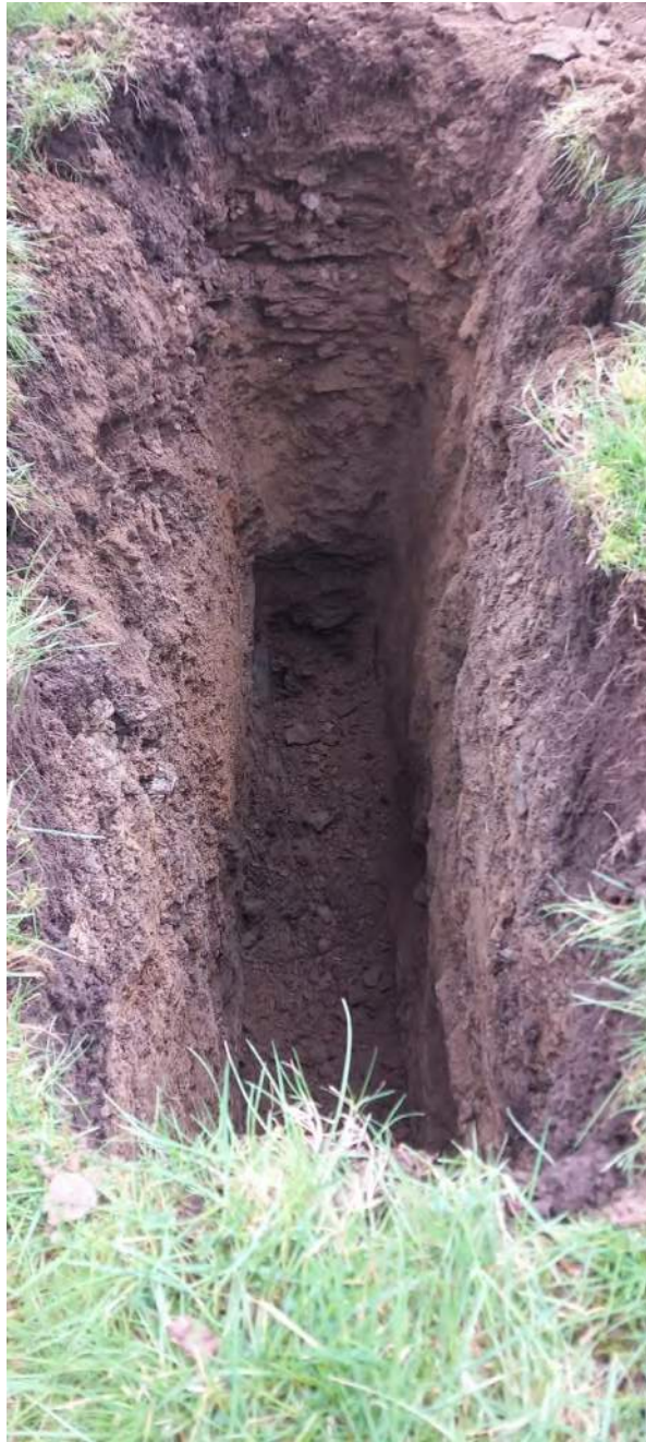
24/02/26 Photo 36 SA202. width 600mm x length 1800mm Topsoil 0.3m over subsoil to 0.4m over laminated siltstone bedrock to 1.5m.
