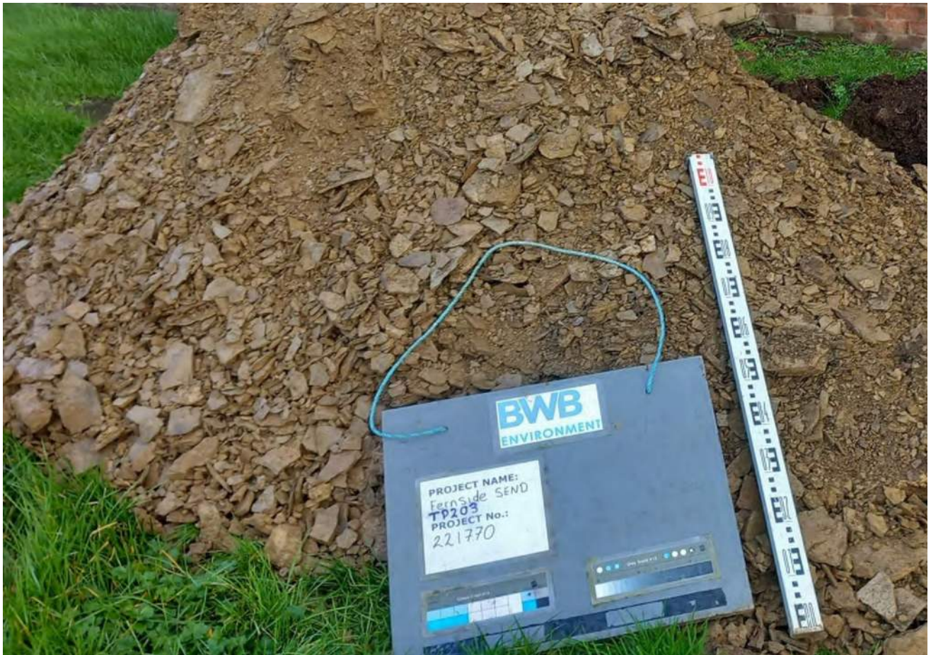
24/02/23 Photo 18 TP203. Arisings weathered thinly laminated siltstone bedrock.
