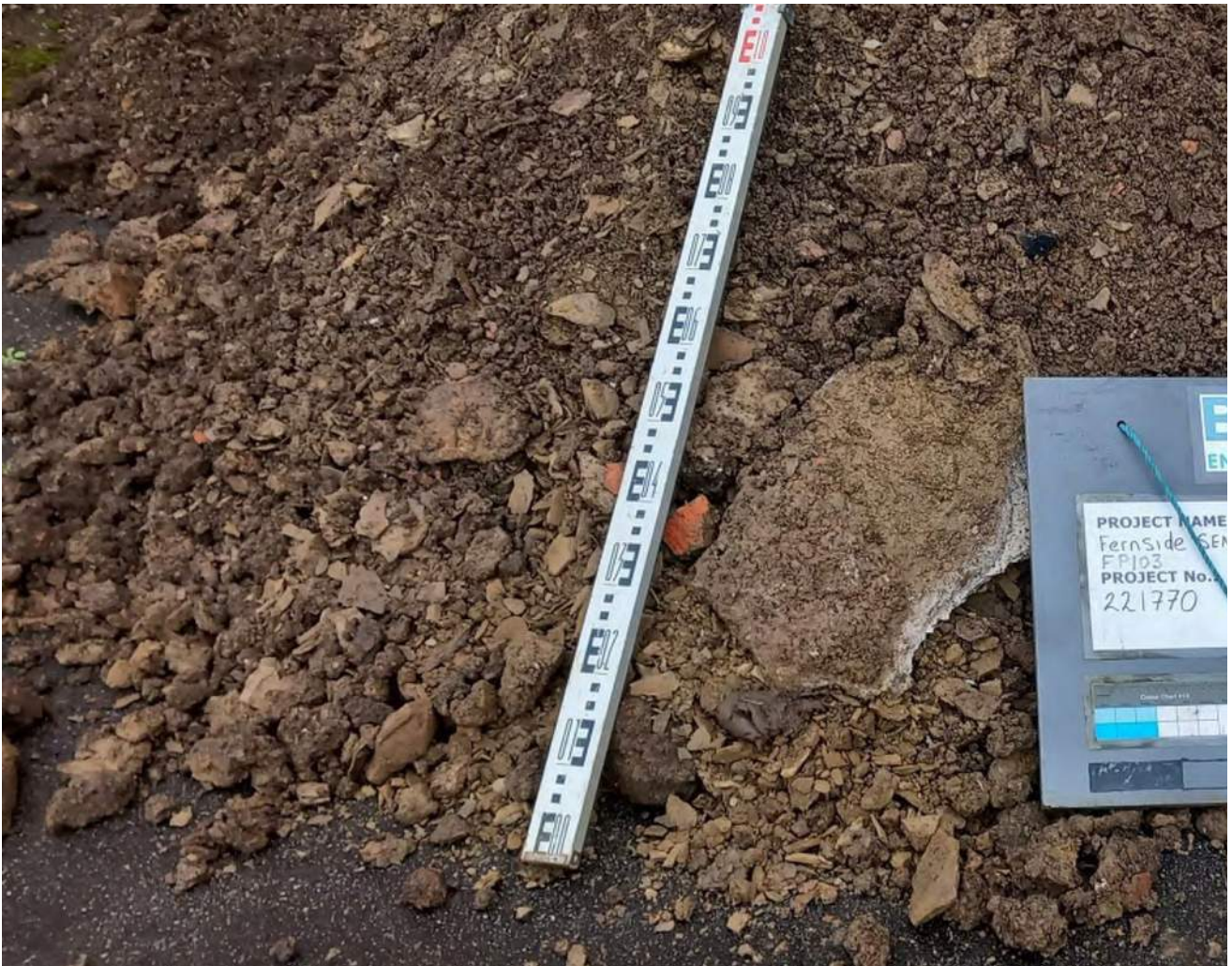
24/02/22 Photo 6 Looking east. FP103. Made ground fill reworked natural with some brick and concrete.
