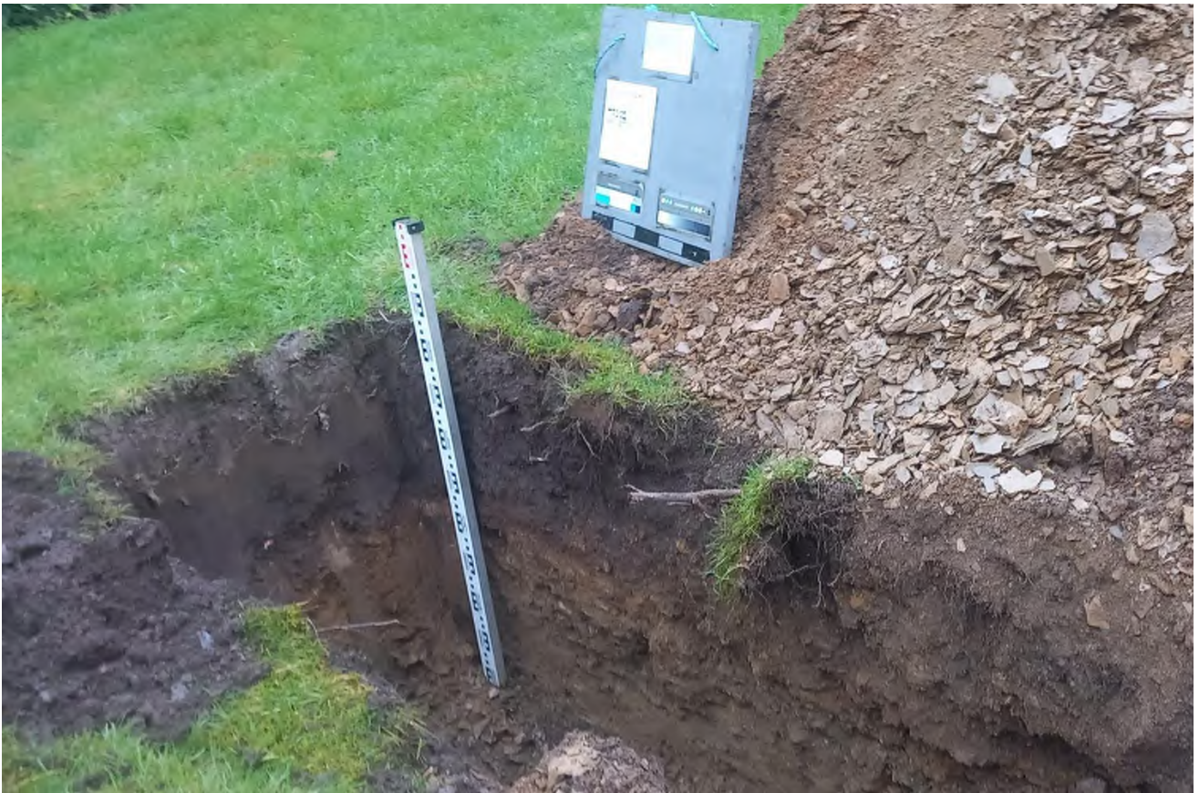
24/02/23 Photo 22 TP201. Topsoil 0.4m over weathered laminated siltstone bedrock
