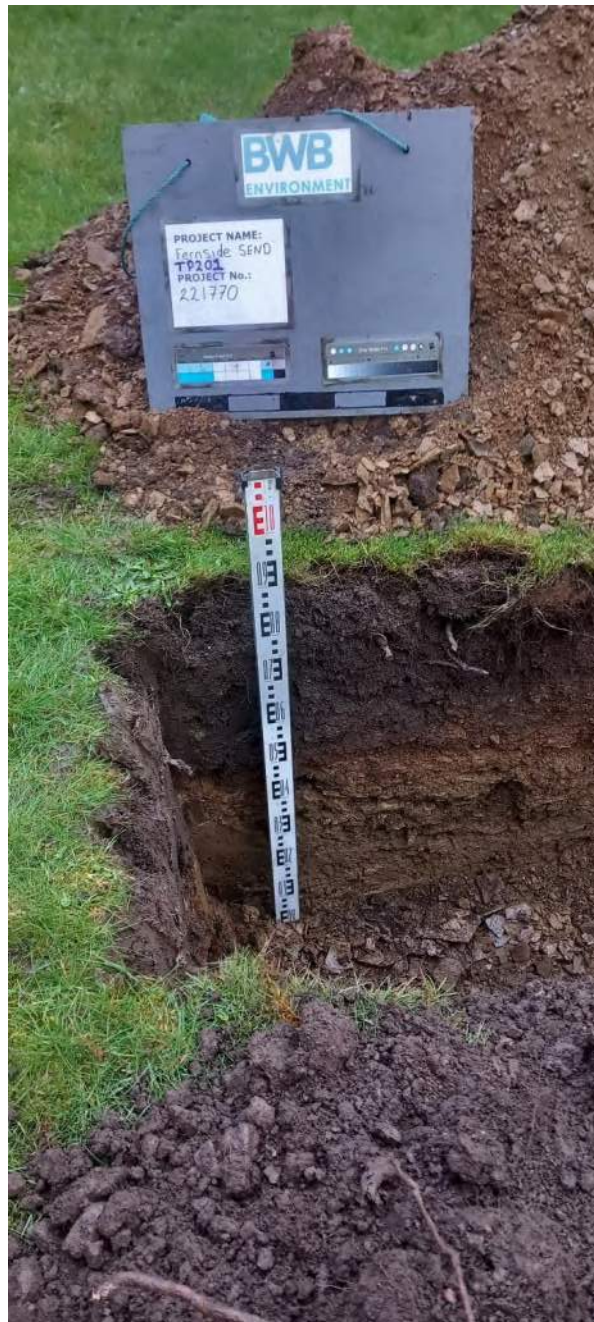
24/02/23 Photo 23 TP201. Topsoil 0.4m over weathered laminated siltstone bedrock
