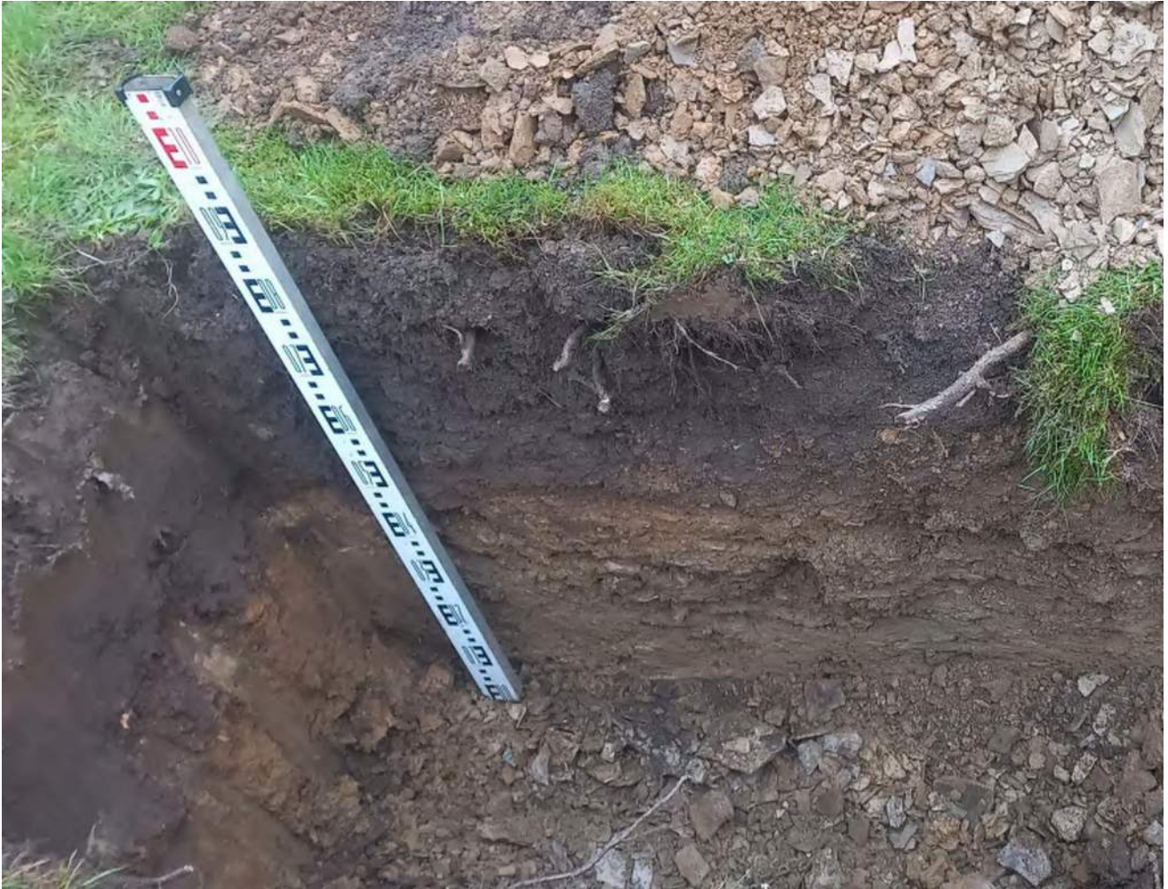
24/02/23 Photo 21 TP201. Topsoil over weathered thinly laminated siltstone bedrock
