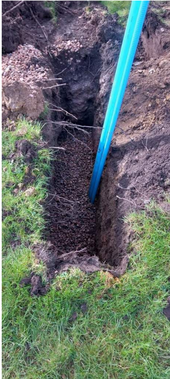
24/02/26 Photo 31 SA204. width 600mm x length 2100mm Gravel from 1.1m to 2.0m depth.
