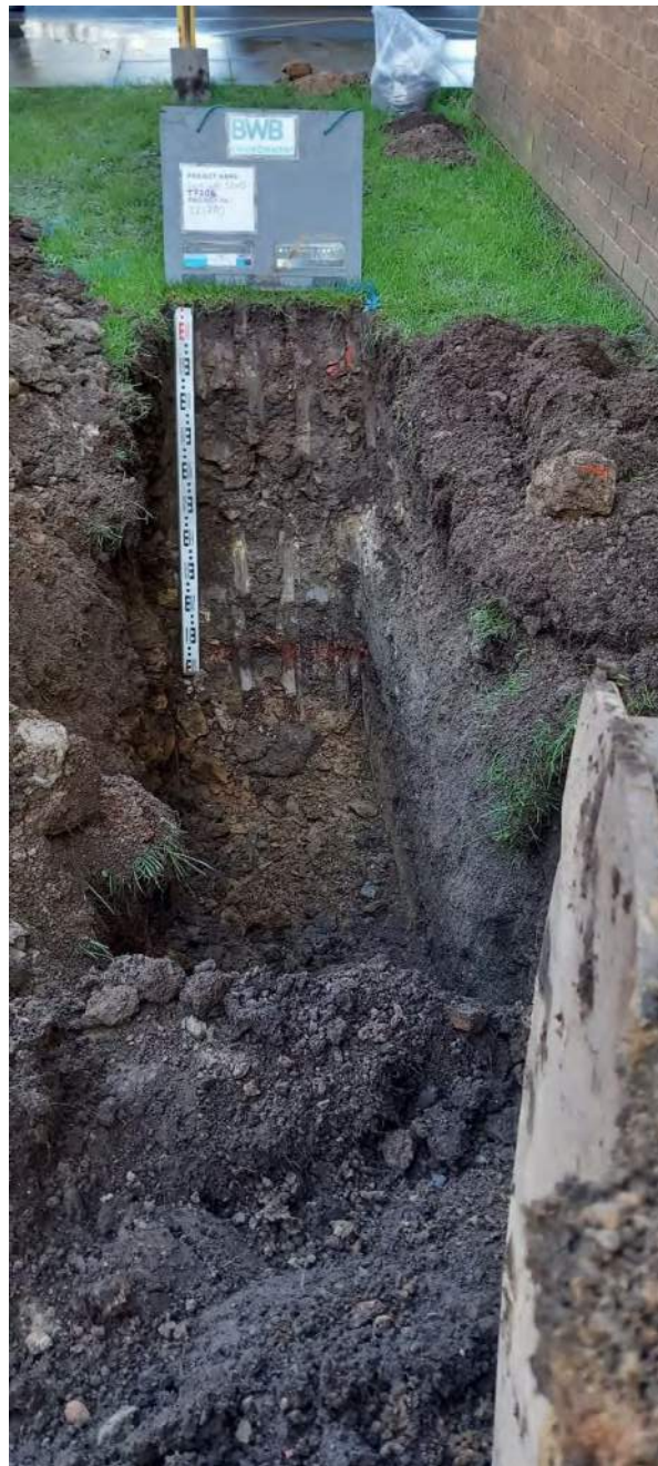
24/02/23 Photo 26 TP204. Topsoil 0.2m over gey made ground (gravelly clay with demo brick and concrete) over compact red shale 0.9m over stiff subsoils 1.1m and weathered laminated siltstone bedrock 1.2m.
