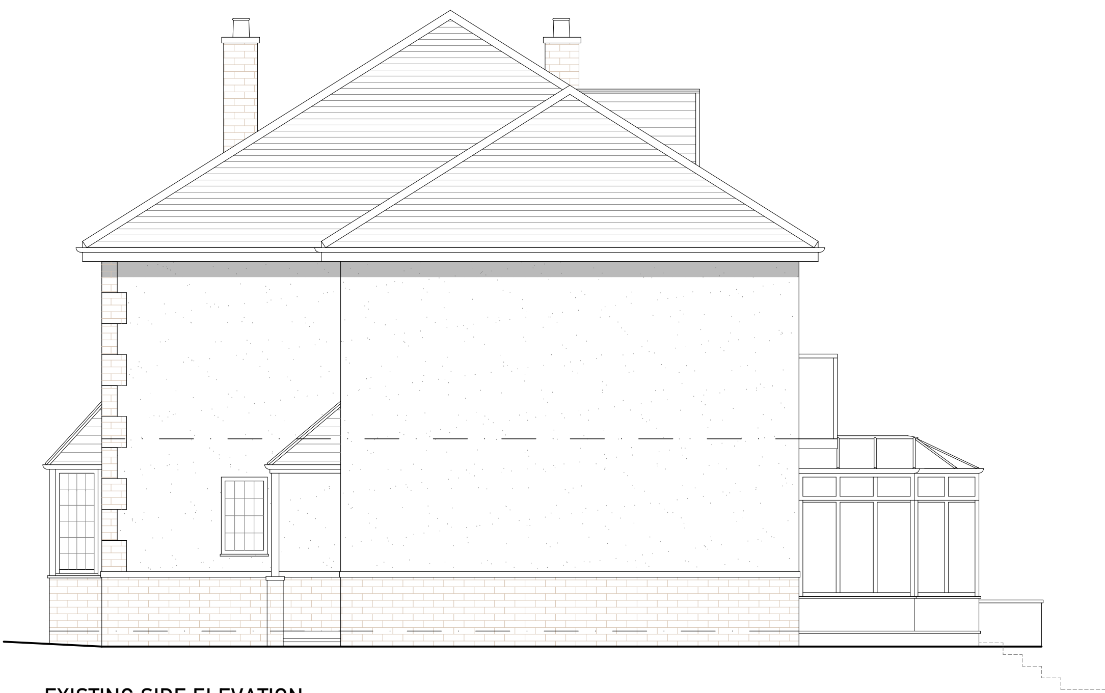
EXISTING SIDE ELEVATION Scale 1:50 at A1
