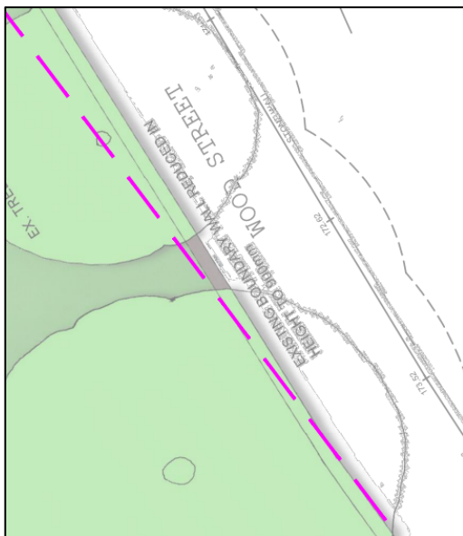
Figure 8 – Splay being impeded by wall (Source ATTP Appendix C HS April 2024)
