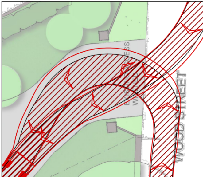
Figure 14 – Swept paths by vehicles entering the site do not leave sufficient space for a vehicle to wait to exit whilst a vehicle enters the site ( Source ATTP Appendix B HS April 2024).
