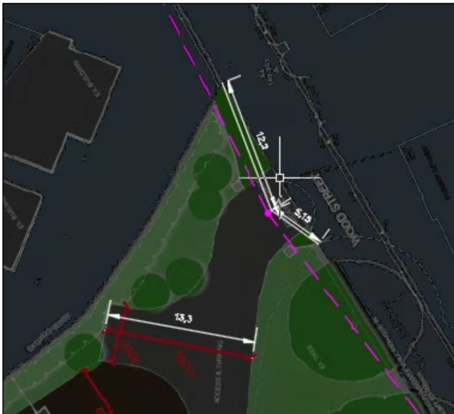
Figure 11 – ATTP PDF Appendix C taken into CAD, (scaled to suit detailed dimension 13.3m.)
