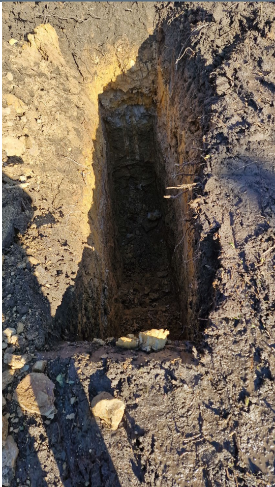
SA01 – Clay below topsoil, sandstone at base.
