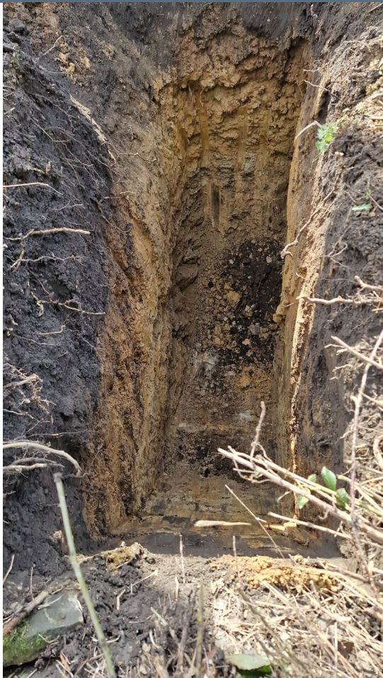
TP03 – Clay below topsoil. Sandstone at base.
