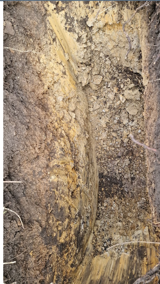
TP01 – Clay below topsoil. Sandstone at base.
