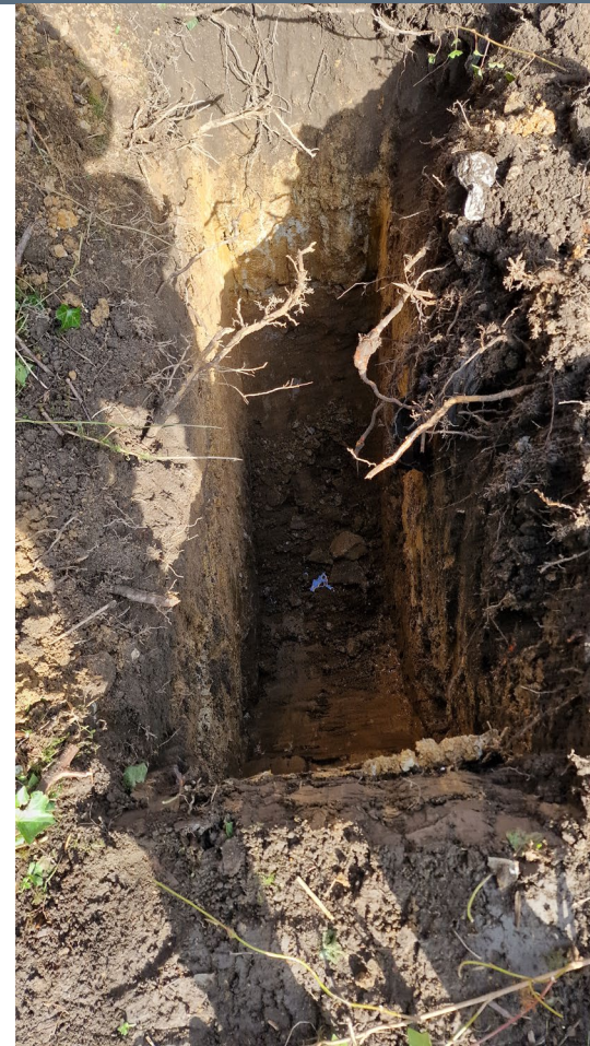
TP07 – Clay below topsoil with sandstone at the base. Groundwater pooling at base.
