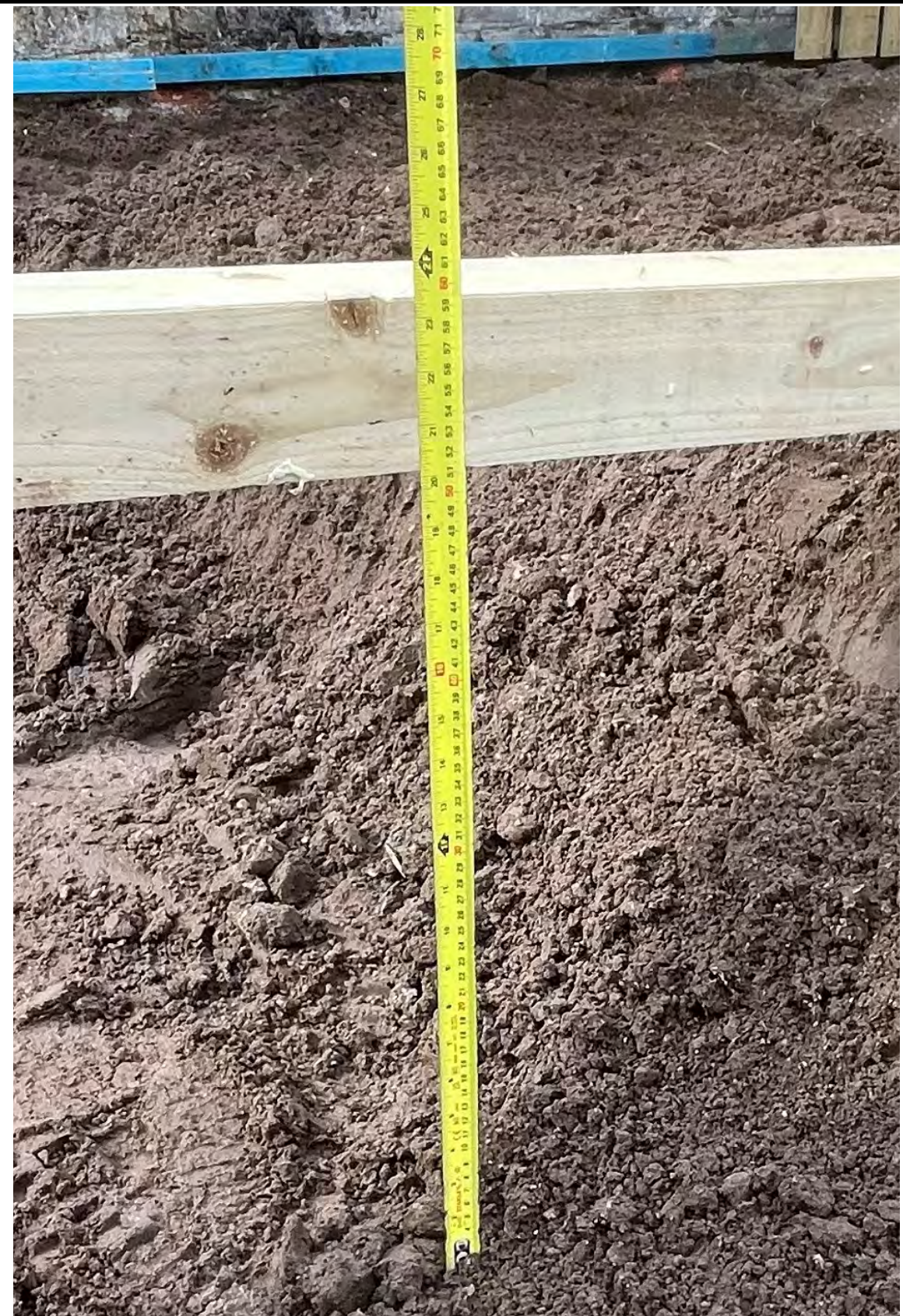
Photo 2: Client Photograph 17.04.24. 500mm of topsoil above capillary break.
