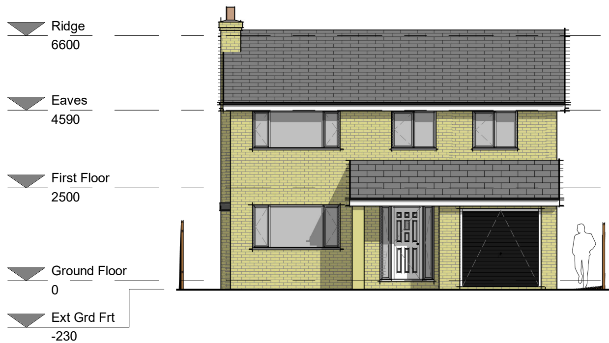
Front Elevation (NE Facing) 1 : 100
