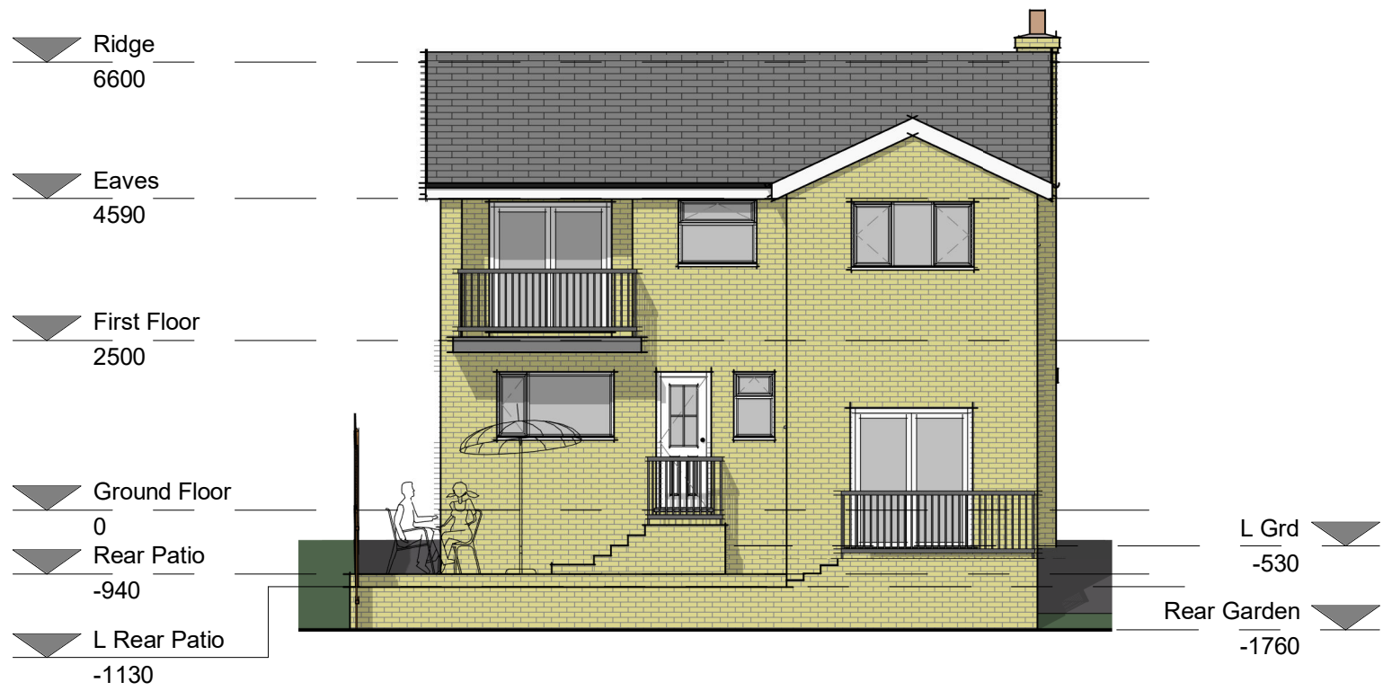
Rear Elevation (SW Facing) 1 : 100
