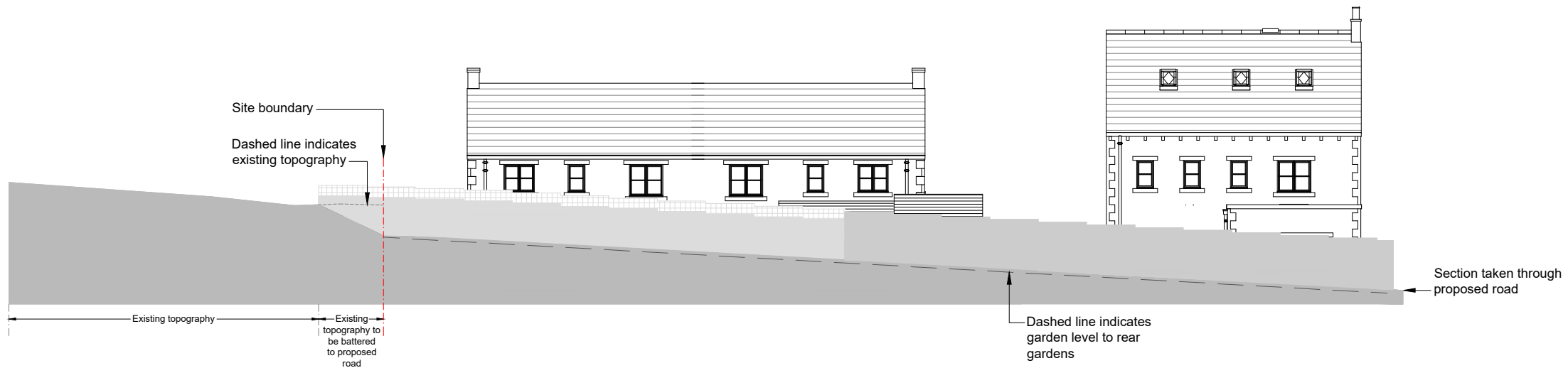
Section 5 - 5 No turning head constructed 1:200
