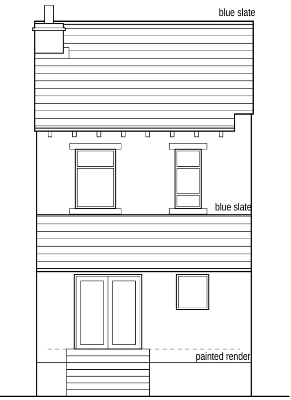
Existing rear/west facing elevation (1:100)
