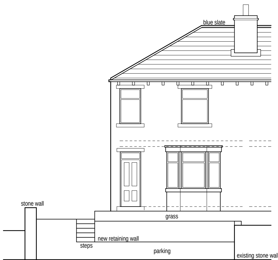
Proposed front/north facing elevation from Manchester Road (1:100)
