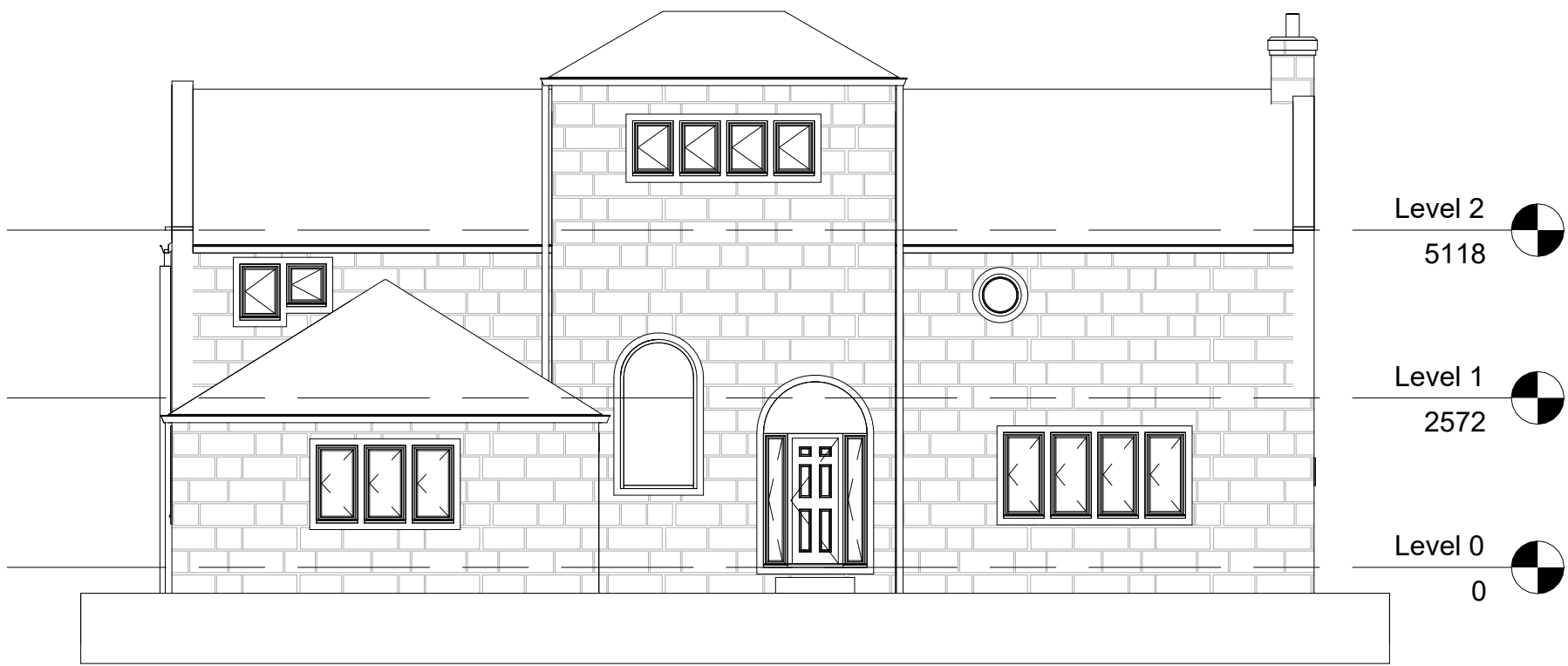
Front Elevation - West 1 : 100
