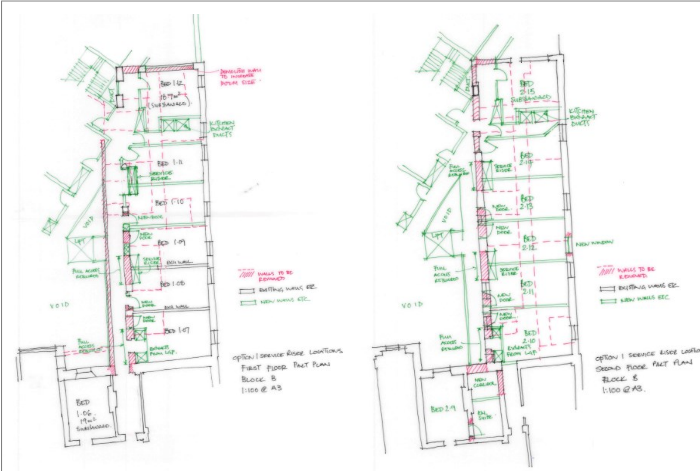
Option 1 for redevelopment with service risers shown and the impact on First and Second Floors
