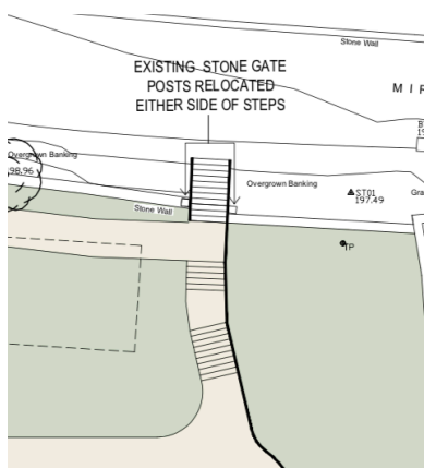
New location of Gate Posts A
