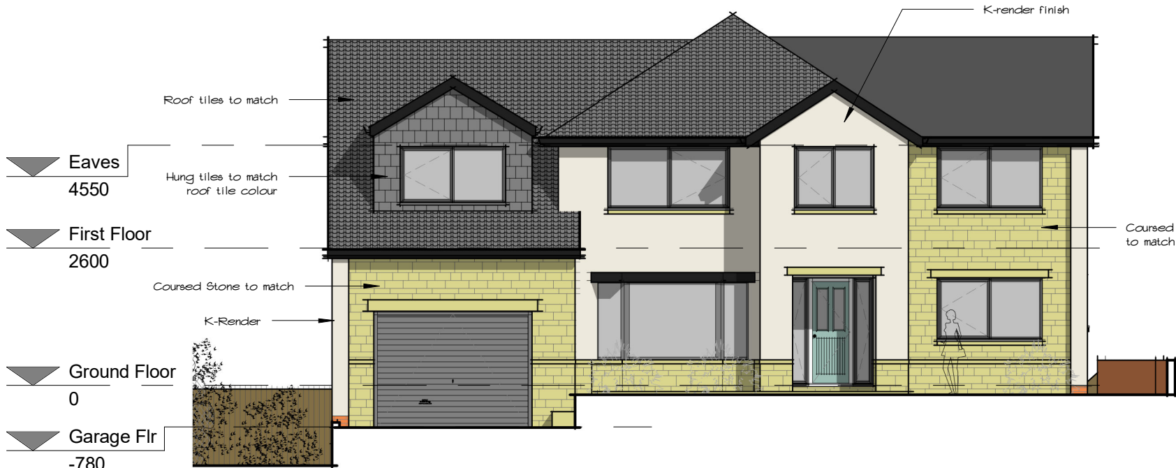
Front Elevation (East Facing) 1 : 100
