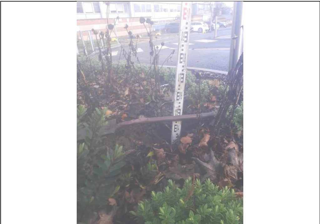
Plate 15: MTP305 Depth check showing 450 mm clean cover.
