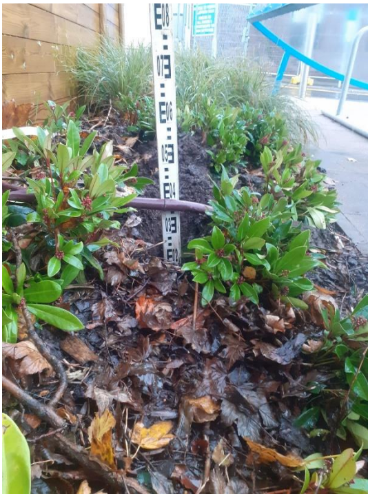
Plate 3: MTP301 Depth check showing 400 mm clean cover.
