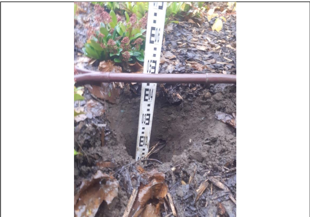
Plate 10: MTP303 Depth check showing 475 mm clean cover.
