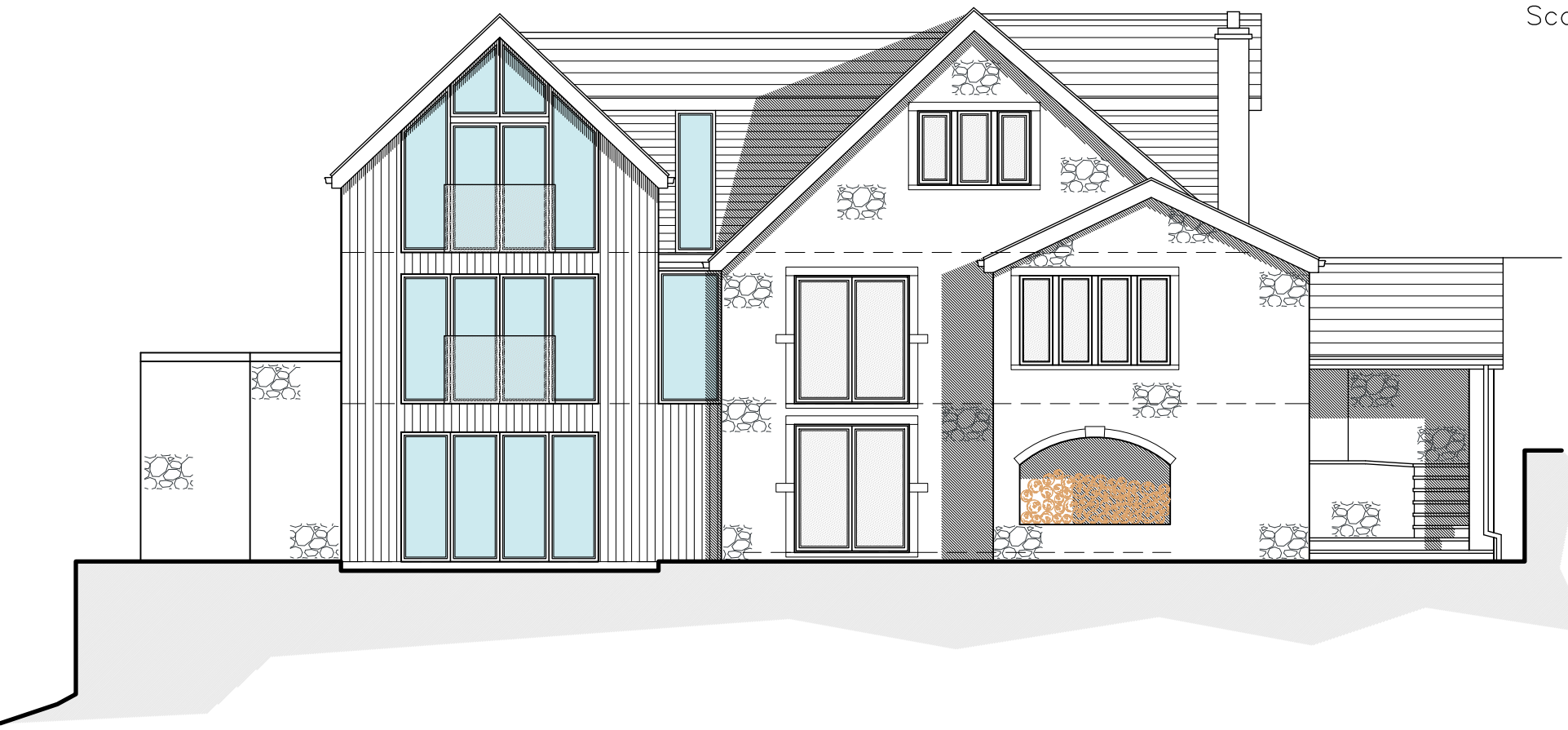
Proposed North East Facing Rear Elevation Scale 1:100
