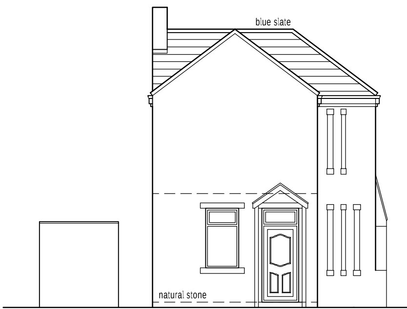
Existing rear elevation (1:100)
