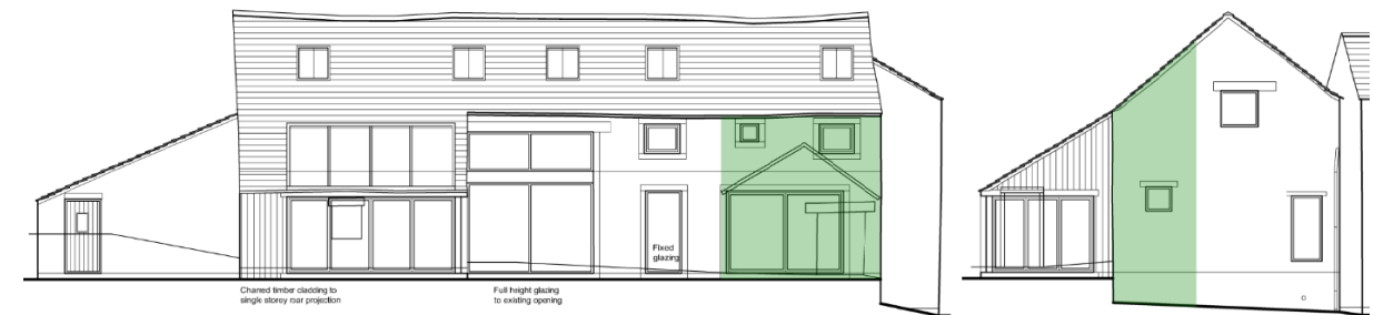
Figure 20 East (left) & north (right) elevations of Stone Barn C with areas of wall to be rebuilt indicated green.
