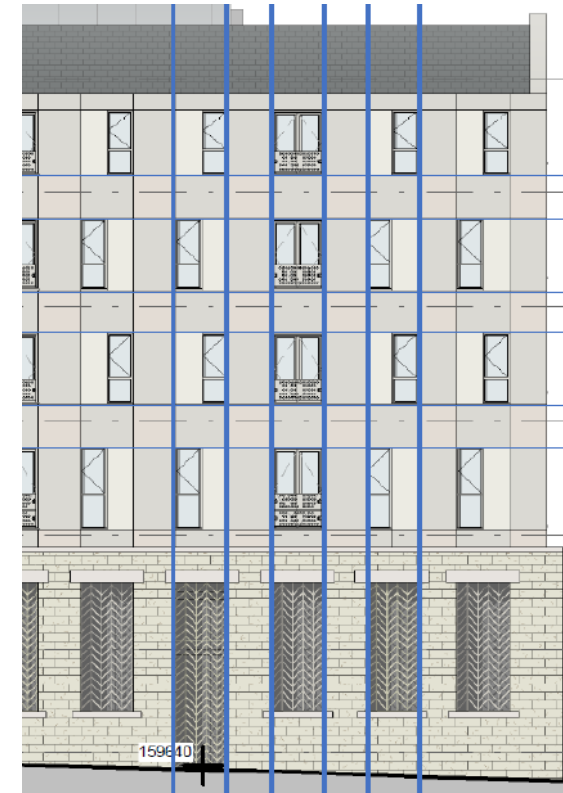
Diagram Extract from Triangle's Window Strategy analysis detailing various acoustic/ heritage/ overheating constraints.
