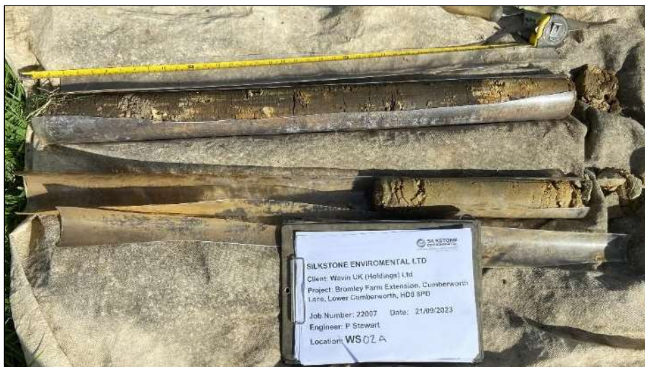
Photo 6: WS02A – Recovered soil cores following penetration to sampler refusal at 1.40m begl (depth progressing from left to right and top to bottom).
