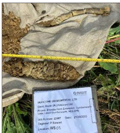
Photo 15: WS05 – Recovered soil core (bottom) and SPT split spoon sample (top) following penetration to sampler refusal at 1.45m begl (depth progressing from left to right and bottom to top).
