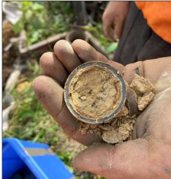
Photo 15: WS05 – Close up of weathered sandstone at the base of the exploratory hole.
