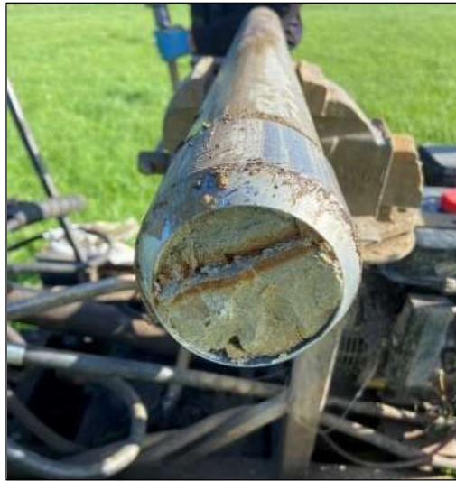
Photo 7: WS02 – Close up of the weathered siltstone at the base of the exploratory hole.
