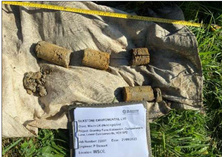
Photo 5: WS02 – Recovered soil core following penetration to sampler refusal at 1.20m begl (depth progressing from left to right and top to bottom).
