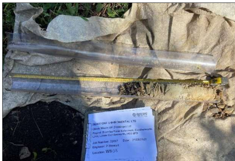
Photo 9: WS03 – Recovered soil core following penetration to sampler refusal at 1.00m begl (depth progressing from left to right).
