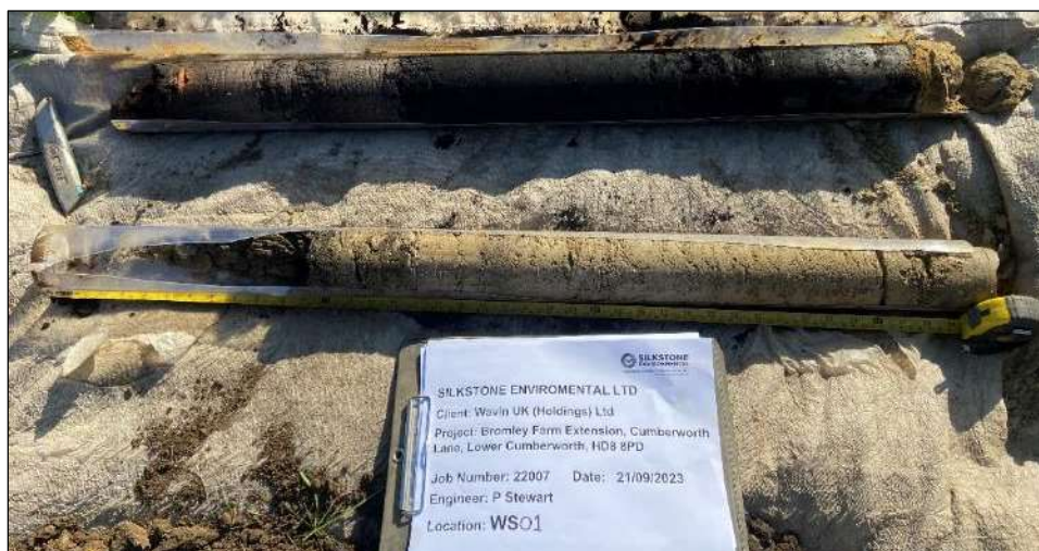
Photo 3: WS01 – Recovered soil core following penetration to sampler refusal at 2.80m begl (depth progressing from left to right and top to bottom).
