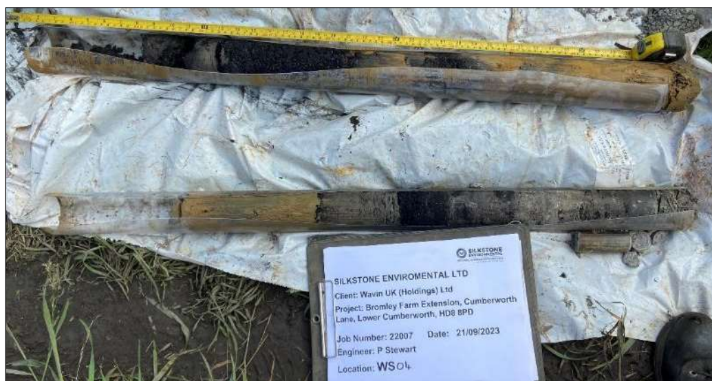
Photo 12: WS04 – Recovered soil cores following penetration to sampler refusal at 2.70m begl (depth progressing from left to right and top to bottom).
