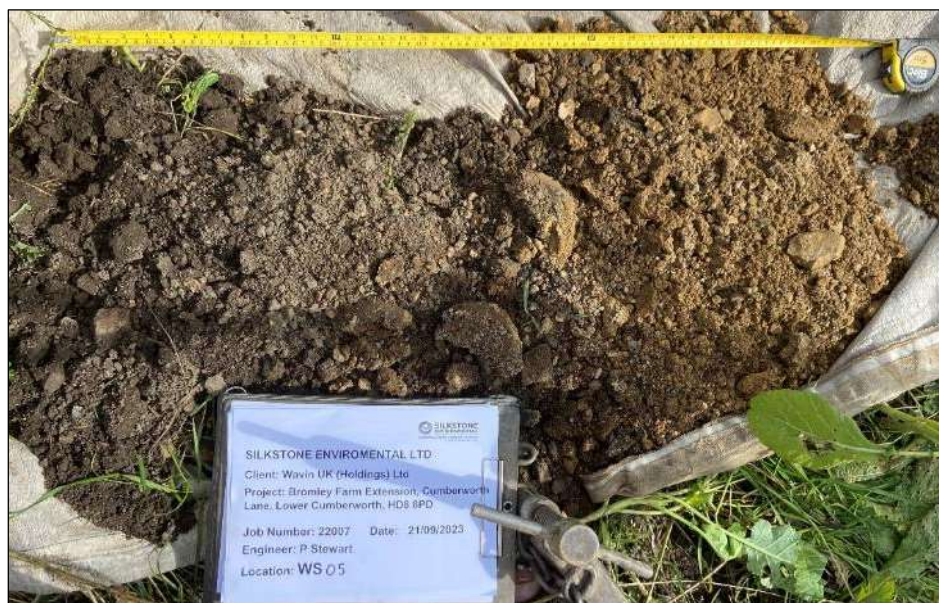
Photo 14: WS05 – Made Ground (Topsoil) and natural soil arisings from hand dug inspection pit (depth progressing from left to right).
