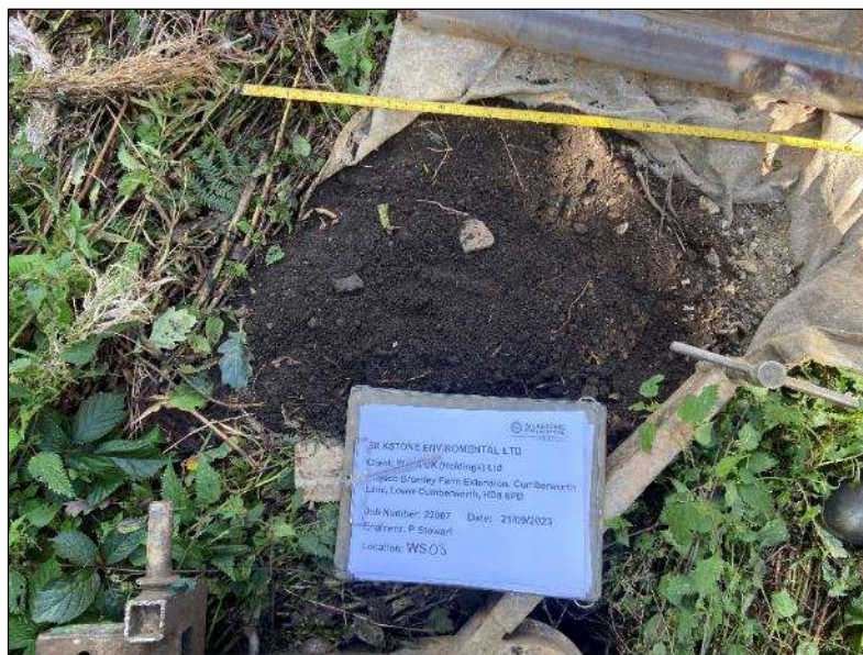
Photo 8: WS03 – Made Ground (Topsoil) arisings from hand dug inspection pit (depth progressing from left to right).
