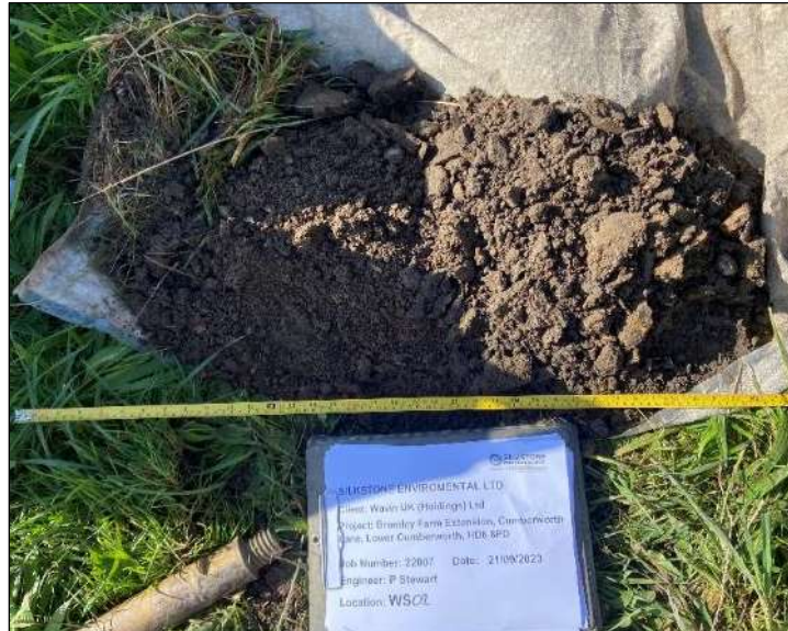
Photo 4: WS02 – Made Ground (Topsoil) arisings from hand dug inspection pit (depth progressing from left to right).
