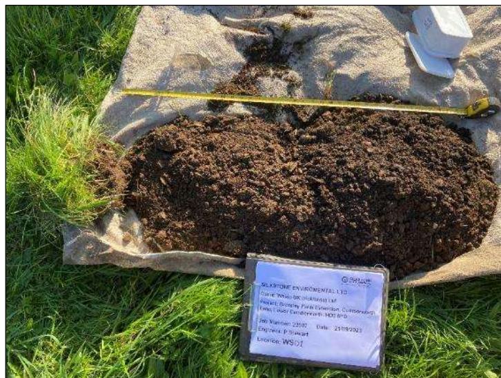
Photo 2: WS01 – Made Ground (Topsoil) arisings from hand dug inspection pit (depth progressing from left to right).
