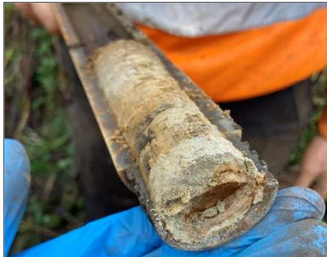
Photo 10: WS03 – Close up of the weathered siltstone at the base of the exploratory hole.
